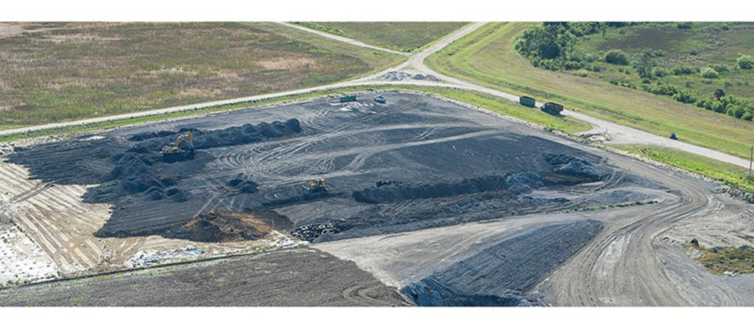
The metals are then separated for recycling. The remaining ash is transported to an ash monofill cell at the Lee/Hendry Landfill.
