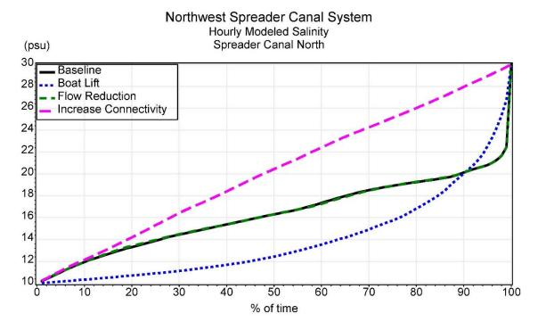
Figure 4-7d. Cumulative Distribution Function for Average Daily Salinity for the NSC North of Gator Slough (Critical Range 10 to 30 ppt)
