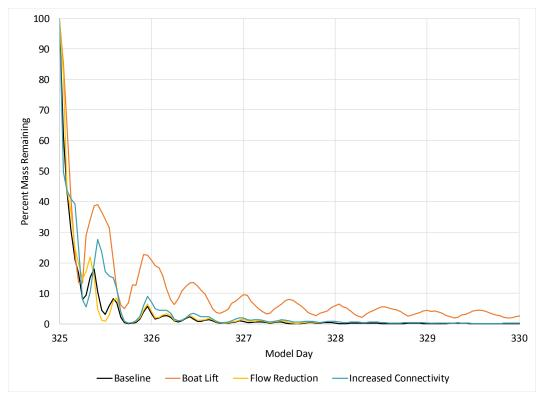
Figure 4-9a. Percent Mass Remaining in Oyster Embayment (high flow condition)
