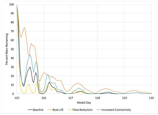
Figure 4-9b. Percent Mass Remaining in Oyster Embayment (low flow condition)
