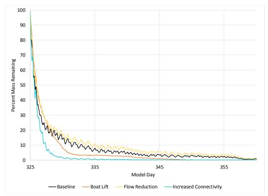
Figure 4-8a. Percent Mass Remaining in Spreader Canal (high flow condition)
