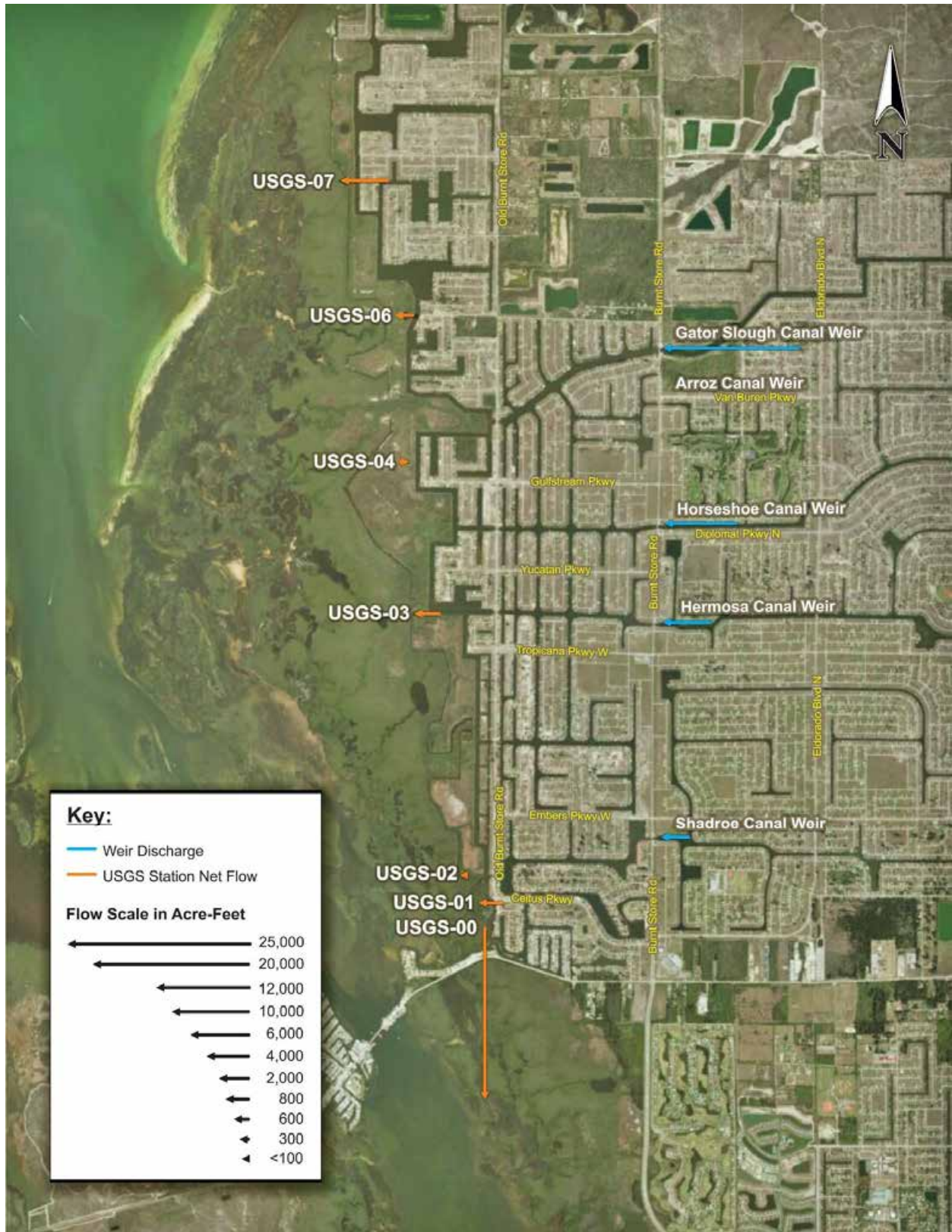
Figure 4-30. Distribution of Net Flows into and out of the NSC for September 2013
