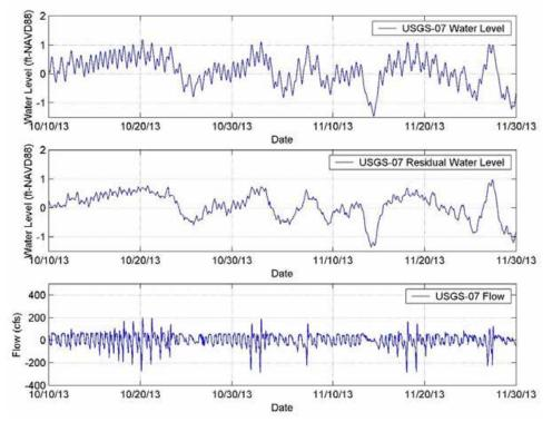
Figure 3-11b. Measured Water Level, Residual Water Level, and Flow at USGS-07, 10/10/13 to 11/30/13(positive = out of NSC, negative = into NSC)
