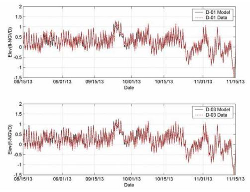
Figure 4-2a. Simulated vs Measured Water Level at Stations D-01 and D-03 (08/15/13 – 11/15/13)
