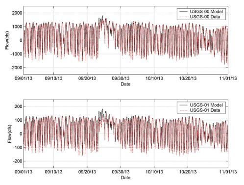
Figure 4-3a. Simulated vs Measured Flow at Stations USGS-00 and USGS-01 (09/01/13 – 11/01/13)
