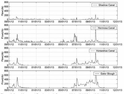
Figure 3-5. Measured Freshwater Inflow over Weirs (9/1/12 to 12/31/15)
