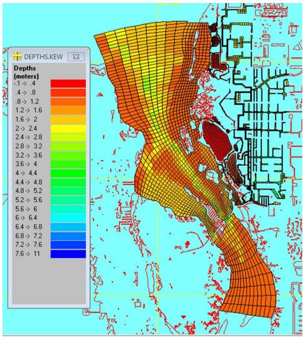
Figure 4-1. Model Grid and Bathymetry
