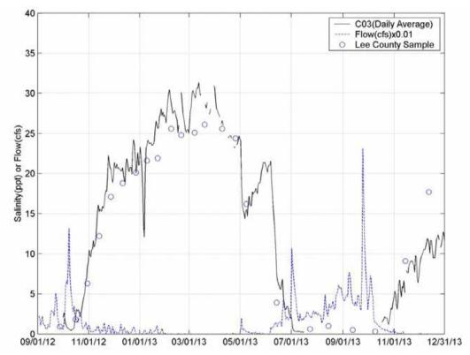
Figure 3-13a. Daily Average/Discrete Salinity versus Flow Over Weirs at C-03
