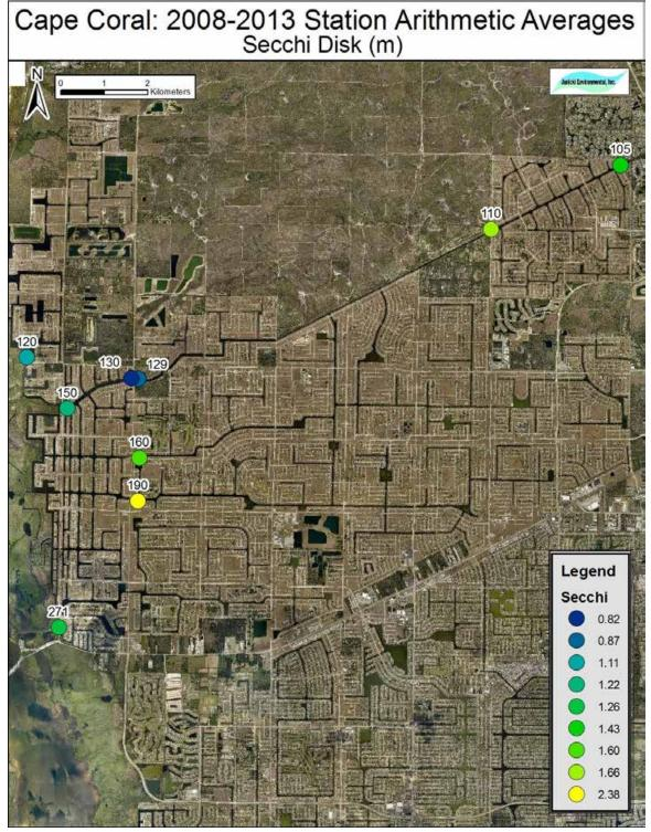
*Figure 5-8.* Arithmetic Average Secchi Disk Visibilities at Cape Coral Stations for Samples Collected between 2008 and 2013
