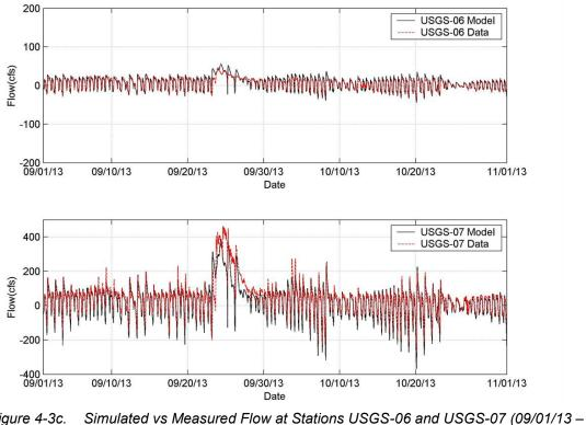
Figure 4-3c. Simulated vs Measured Flow at Stations USGS-06 and USGS-07 (09/01/13 11/01/13)
