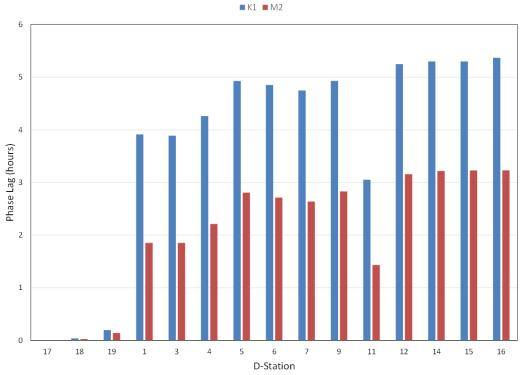
Figure 3-8b. Tidal Harmonic Phase Lag from D-17 by Station
