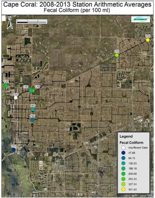
*Figure 5-10.* Arithmetic Average of Fecal Coliform at Cape Coral Stations for Samples Collected between 2008 and 2013 in the NSC
