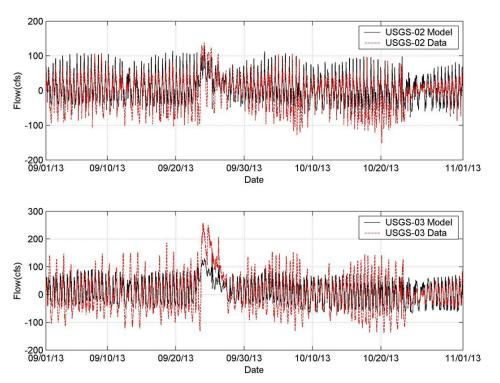
Figure 4-3b. Simulated vs Measured Flow at Stations USGS-02 and USGS-03 (09/01/13 – 11/01/13)
