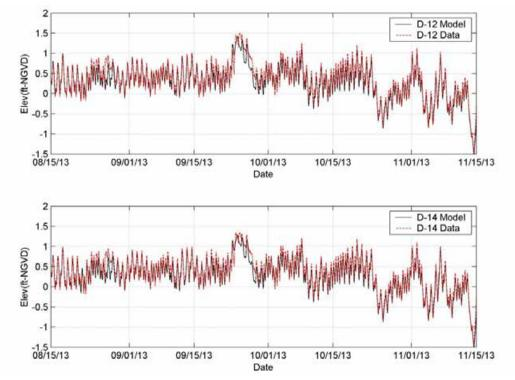
Figure 4-2b. Simulated vs Measured Water Level at Stations D-12 and D-14 (08/15/13 – 11/15/13)
