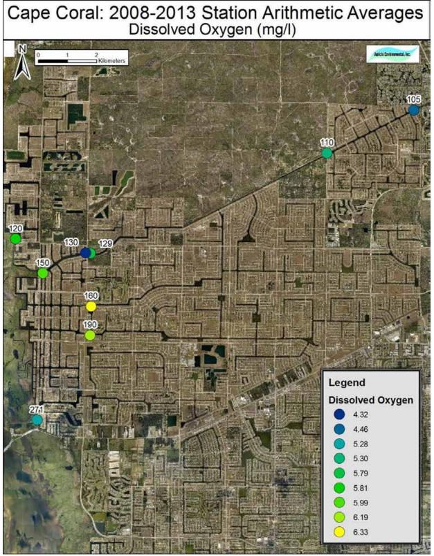
*Figure 5-4.* Arithmetic Average of Surface Dissolved Oxygen at Cape Coral Fixed Station Samples Collected between 2008 and 2013 in the NSC
