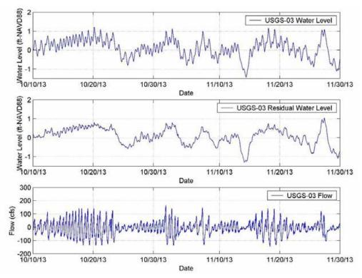
Figure 3-11a. Measured Water Level, Residual Water Level, and Flow at USGS-03, 10/10/13 to 11/30/13 (positive = out of NSC, negative = into NSC)
