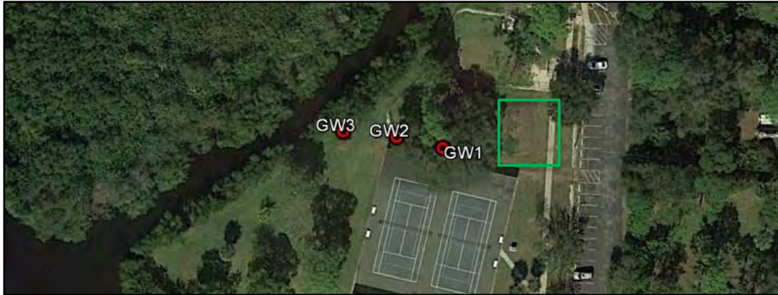
Figure 8. Groundwater monitoring wells (GW1-GW3) in Judd Community Park located within the Hancock Creek watershed on the western side of North Fort Myers, FL; the approximate location of the septic tank drainfield is indicated by the green square.
