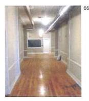
Not Recommended: [66] Interior ductwork has been inappropriately left exposed and unpainted here in this traditionally-finished school entrance hall.
