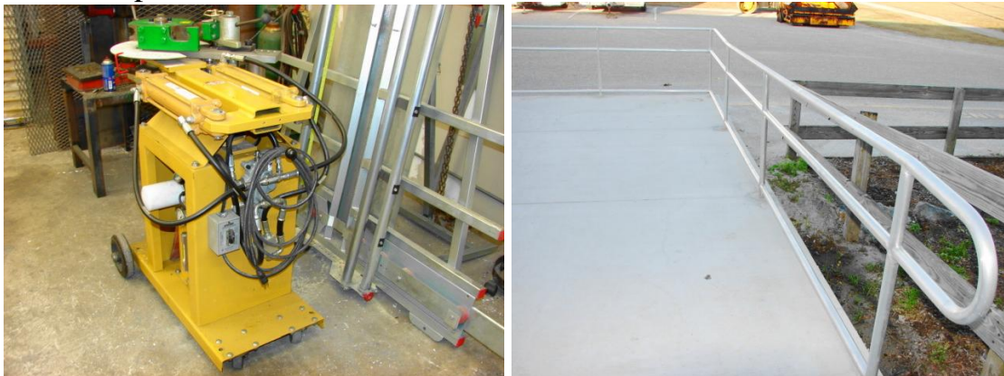
The machine fabricates ADA compliant railings at a fraction of the cost a vendor would charge
