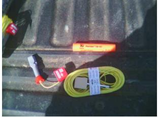
Non-electric detonator and primer cartridge
