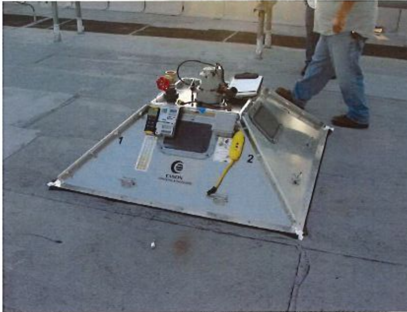
Photo 14 – View of negative pressure chamber testing apparatus. The system creates a vacuum inside the chamber which imparts an upward force on the roofing system. In accordance with test standards, deflection of the roofing system is measured and compared to allowable tolerances. Excessive upward deflection observed prior to achieving the required design pressures, indicates inadequate system securement.
