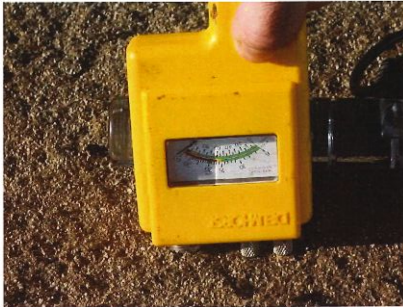
Photo 5 – Moisture meter probes confirmed the presence of high moisture content within the perlite coverboard. We believe this moisture contamination occurred as a result of the membrane split illustrated in the previous photographs.
