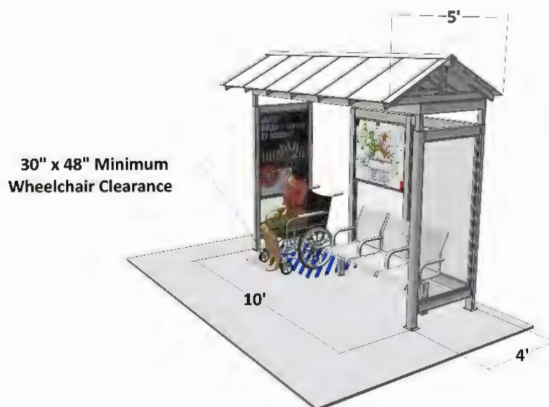
Figure 3.6: Bus Shelter Typical Dimensions
