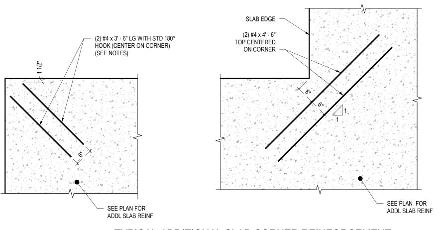
TYPICAL ADDITIONAL SLAB CORNER REINFORCEMENT
