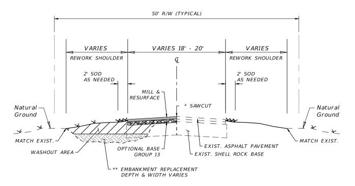
SAWCUT POINT WILL VARY BASED ON LIMITS OF DAMAGE \*\* EMBANKMENT REPLACEMENT MATERIALS SHALL MEET THE REQUIREMENTS OF SECTION 120 OF THE STANDARD SPECIFICATIONS. EXISTING DISPLACED EMBANKMENT MATERIALS CAN BE RE-USED IF THEY MEET THE REQUIREMENTS OF SECTION 120 OF THE STANDARD SPECIFICATIONS.
