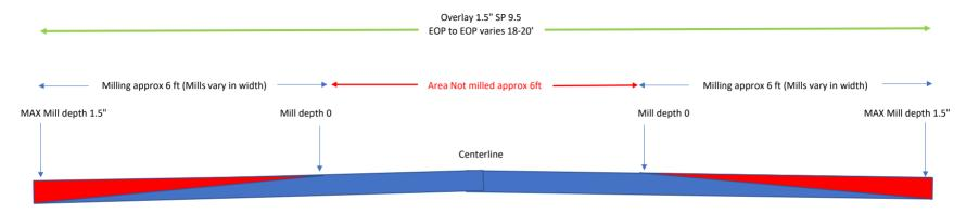
"AC asphalt roads shall be fade milled with a single pass on each side of the roadway from 0 on the centerline side and a 1.5 on low side or at a depth not to damage the existing base."
