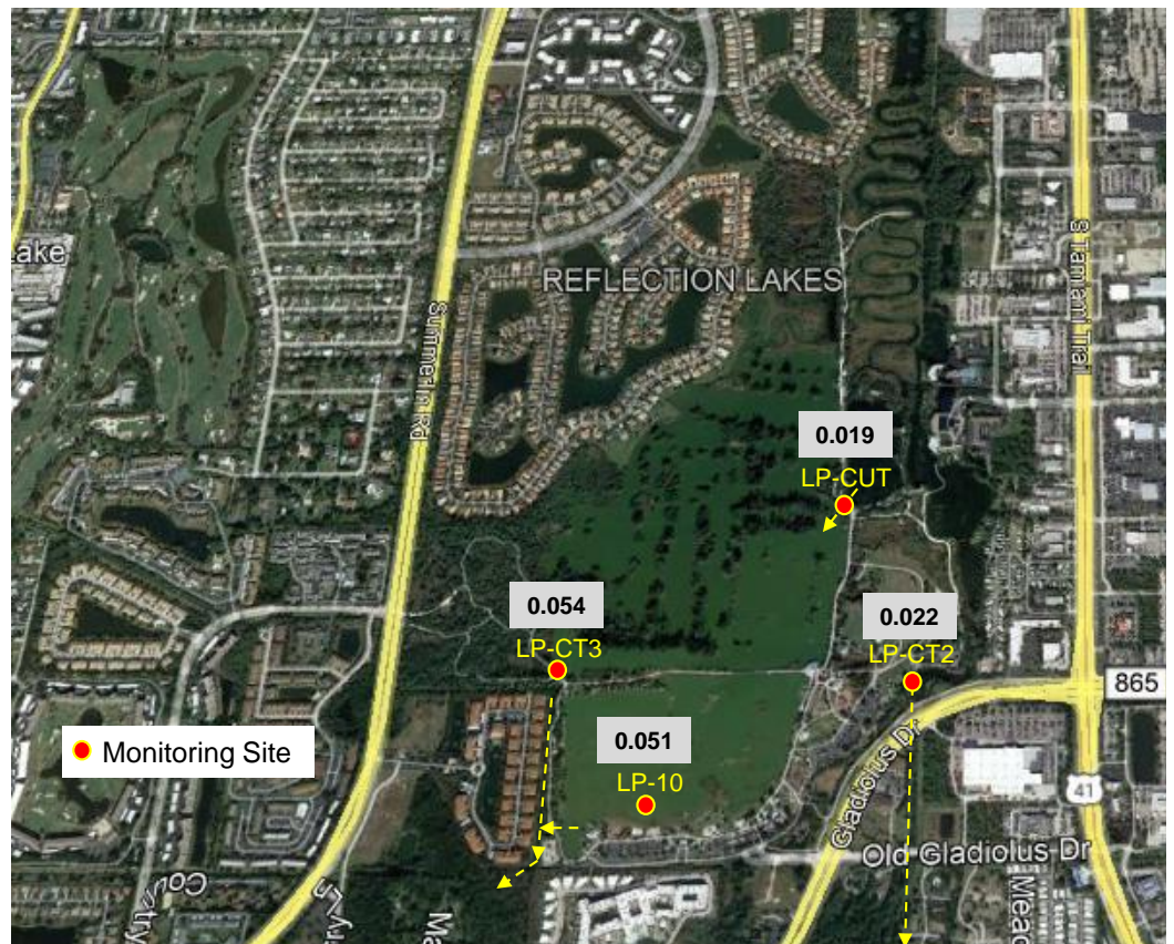
Figure 2-5. Geometric Mean Concentrations of Total Phosphorus (mg/l) at West Lake Monitoring Sites from 2016-2020.
