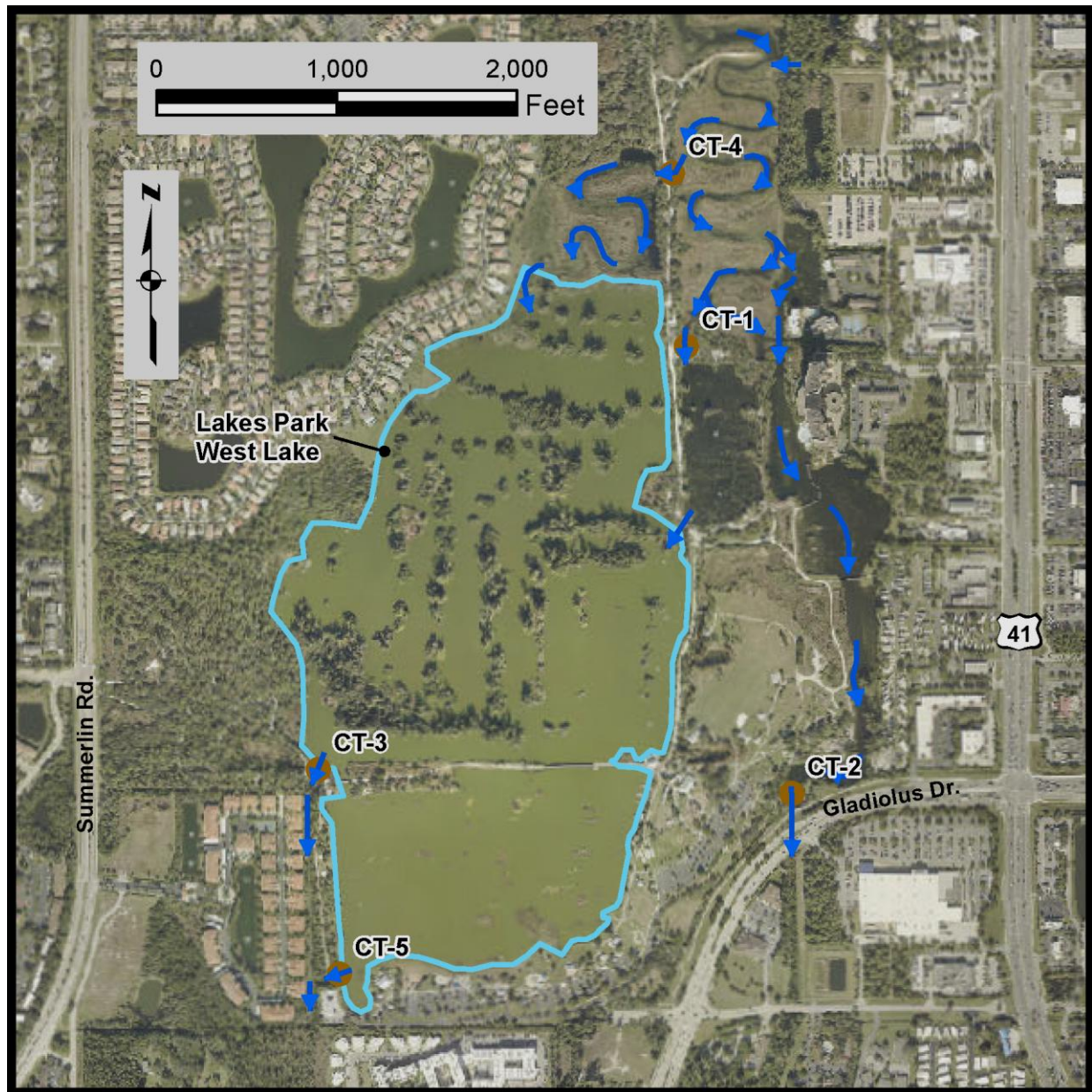
Figure 1-3. Flow Patterns for the Hendry Creek Wetland Treatment System and West Lake.
