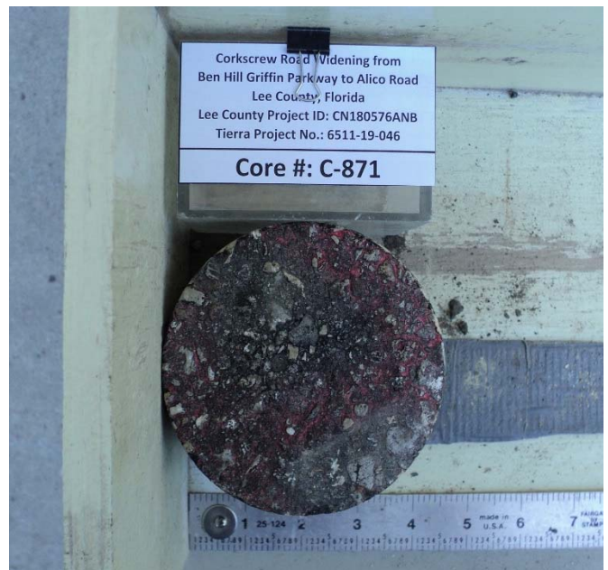
Photograph 27. Top View of Pavement Core C-871
