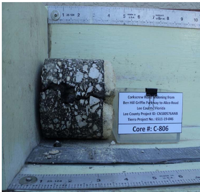
Photograph 8. Side View of Pavement Core C-806
