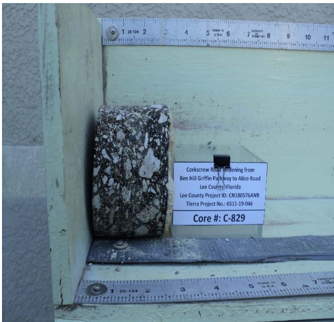
Photograph 14. Side View of Pavement Core C-829
