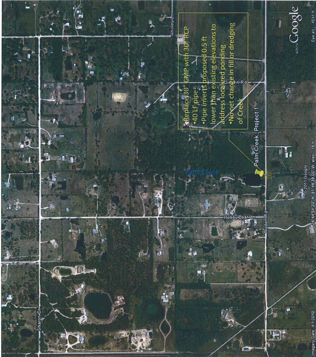
Exhibit A3. Site Plan, Palm Creek Culvert Replacement Please refer to Exhibits 14 "Typical Sections" & 15 "Details" attached for further information.
