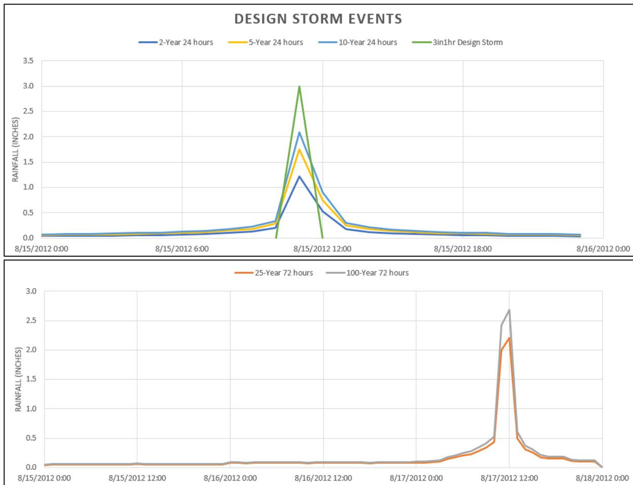
Figure 16. The rainfall intensity curves for the developed into the Design Storm simulations. The short duration events are shown on the top and the long-duration events are shown on the bottom.
