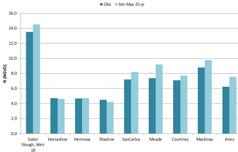
Figure 17. Comparison of 25-yr Design Storm peak stages with a 25-year period of record for observed data. Peak stages at each of the locations in Cape Coral during the Design Storm are similar to max observed values in the 25 year period of record.
