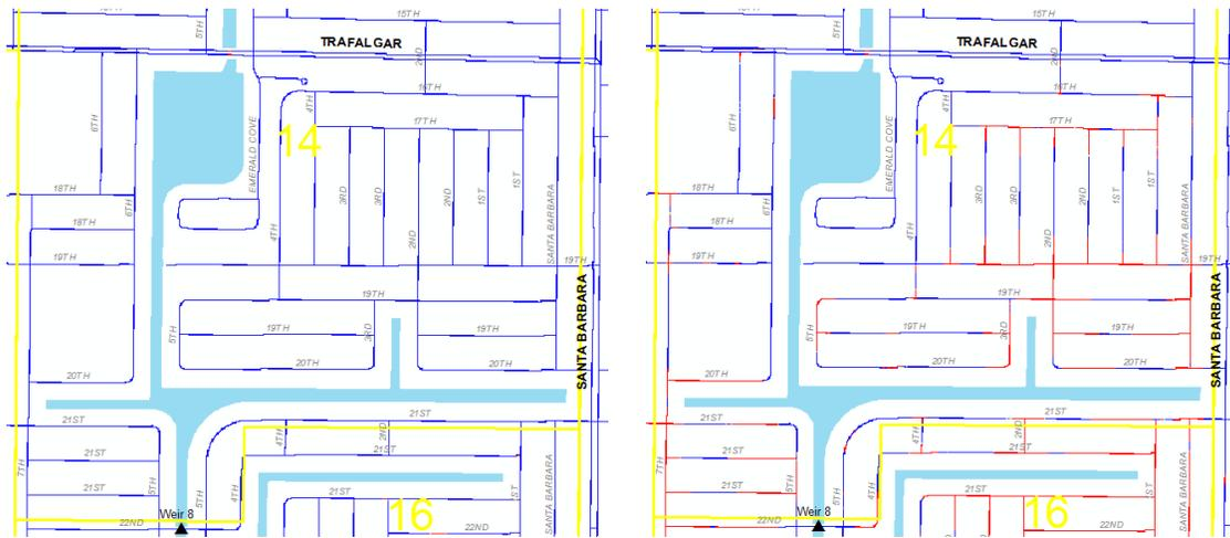
Figure 25. Basin 14 road flooding (red lines) for the “All Gates Down” scenario in the left image and the “Fully Up” scenario in the right image.
