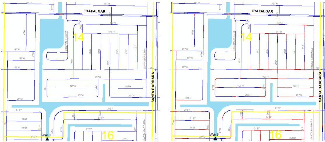
Figure 25. Basin 14 road flooding (red lines) for the "All Gates Down" scenario in the left image and the "Fully Up" scenario in the right image.
