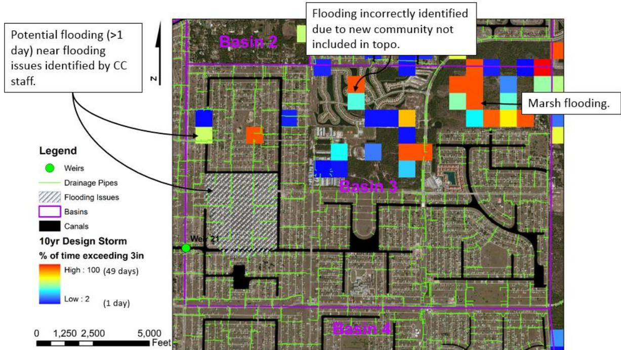
Figure 21. Secondary flooding in Basin 3. The colored squares indicate the percent of time that there is more than 3 inches of water during the 10 year Design Storm simulation.
