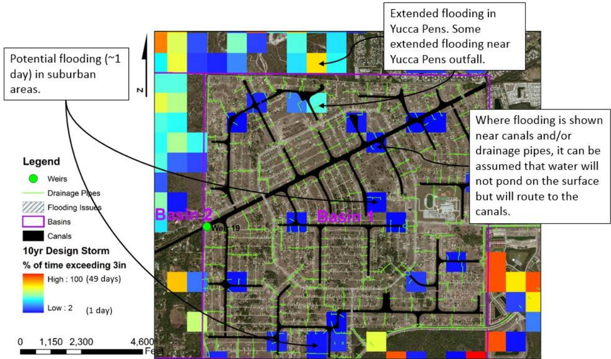
Figure 20. Secondary flooding in Basin 1. The colored squares indicate the percent of time that there is more than 3 inches of water during the 10 year Design Storm simulation.
