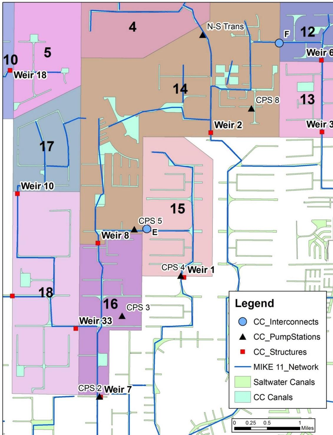
Figure 14. Basins and structures which are critical for maintaining a balanced water budget for the City of Cape Coral south of Pine Island Rd. Basin 12, 13, 14, 15, and 16 all receive flows from the N-S transfer station and are part of a larger water budget termed the Southern Basins.
