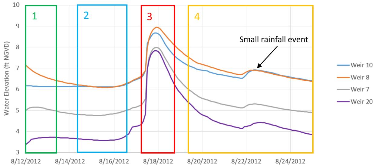
Figure 30. Depiction of the different phases of Basin drainage during a 25 yr Design Storm
