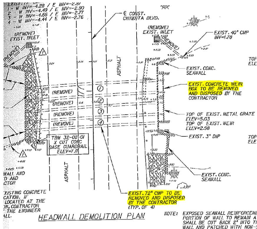
Figure 24. Chiquita Blvd Improvement plans indicate that the existing culverts and Weir 20 will be removed and disposed of and then replaced with structures of the same or similar dimensions and elevations.
