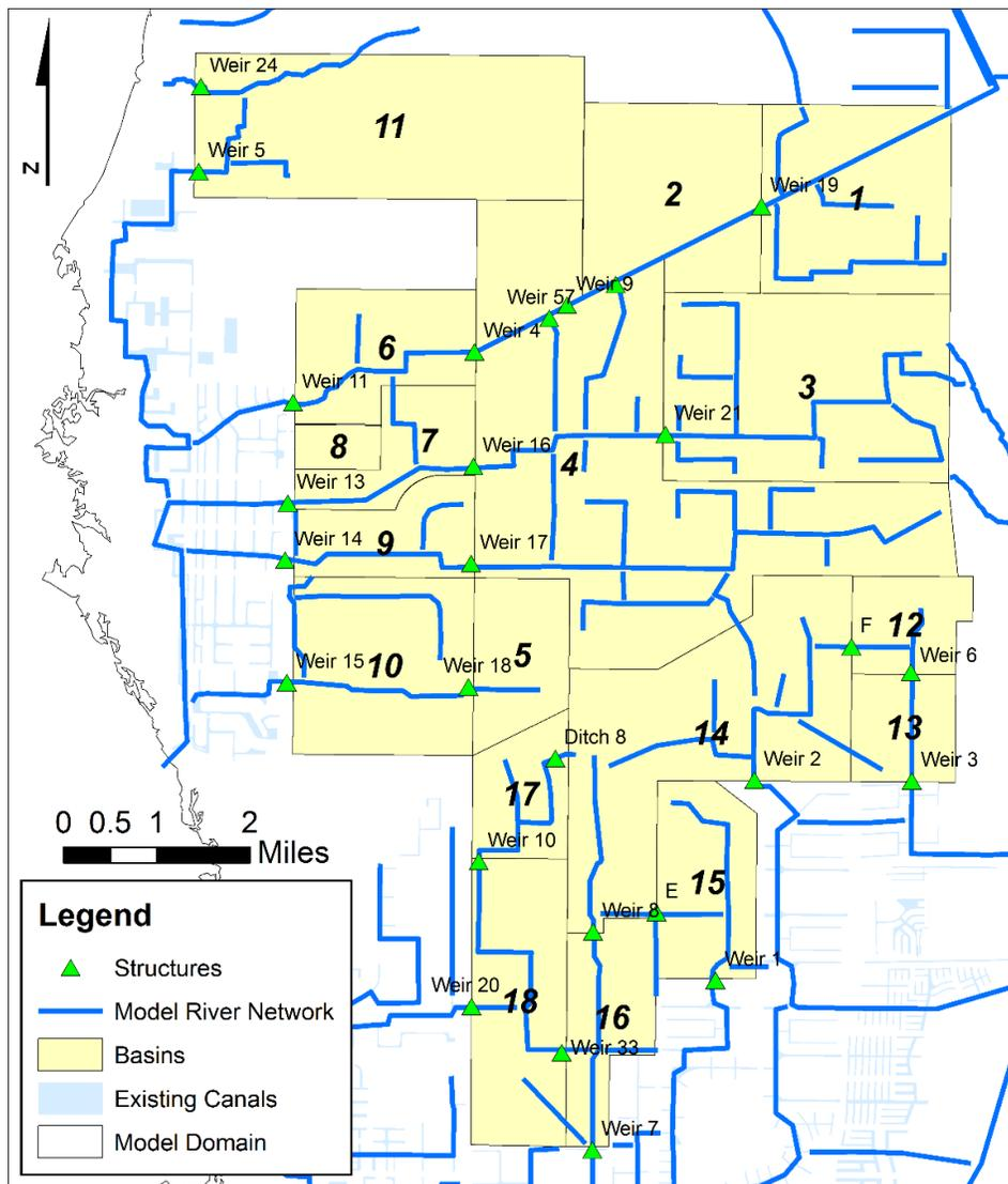
Figure 2. Canal network with locations of structures within the City of Cape Coral.
