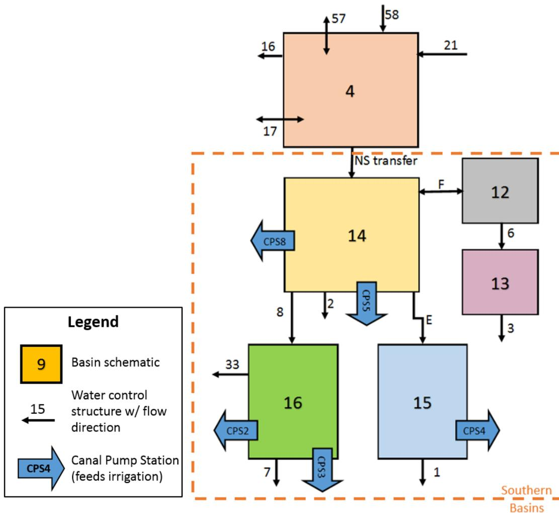
Figure 12 Canal Basins water balance schematic.
