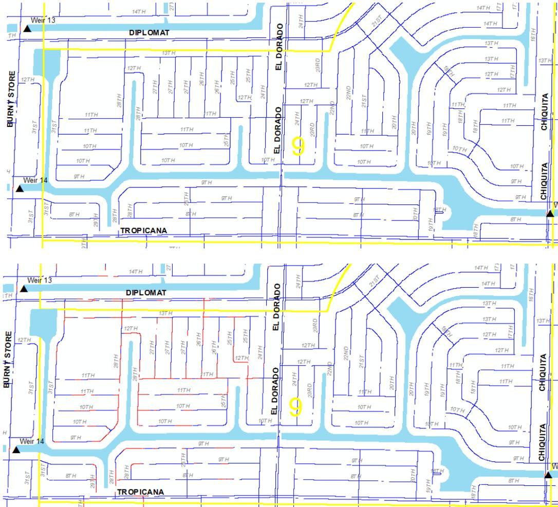
Figure 26. Basin 9 road flooding (red lines) for the “All Gates Open” scenario in the top image and the “Fully Up” scenario on the bottom.
