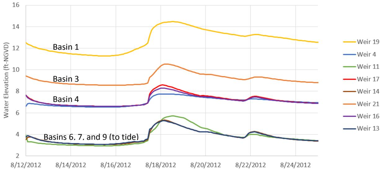
Figure 28. Hydrographs for the Upper Basins of Cape Coral for the first 13 days of the 25yr Design Storm simulation with Existing Conditions.
