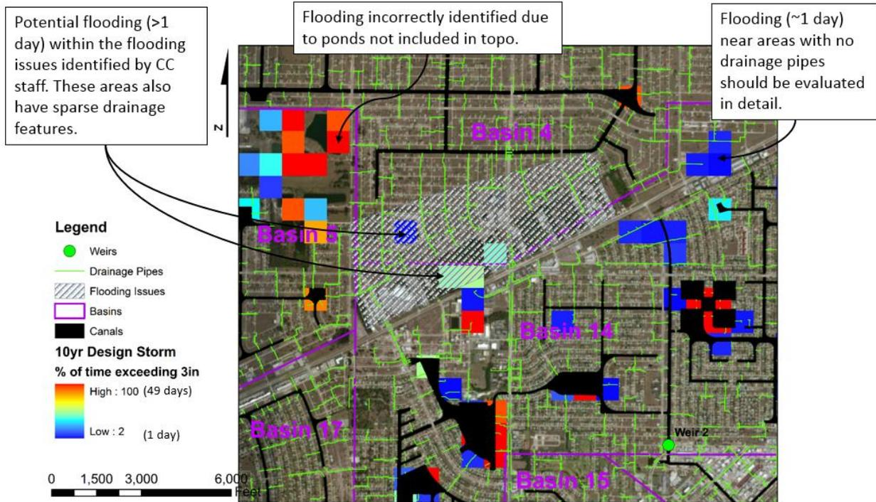
Figure 22. Secondary flooding in Basin 4 and 14. The colored squares indicate the percent of time that there is more than 3 inches of water during the 10 year Design Storm simulation.
