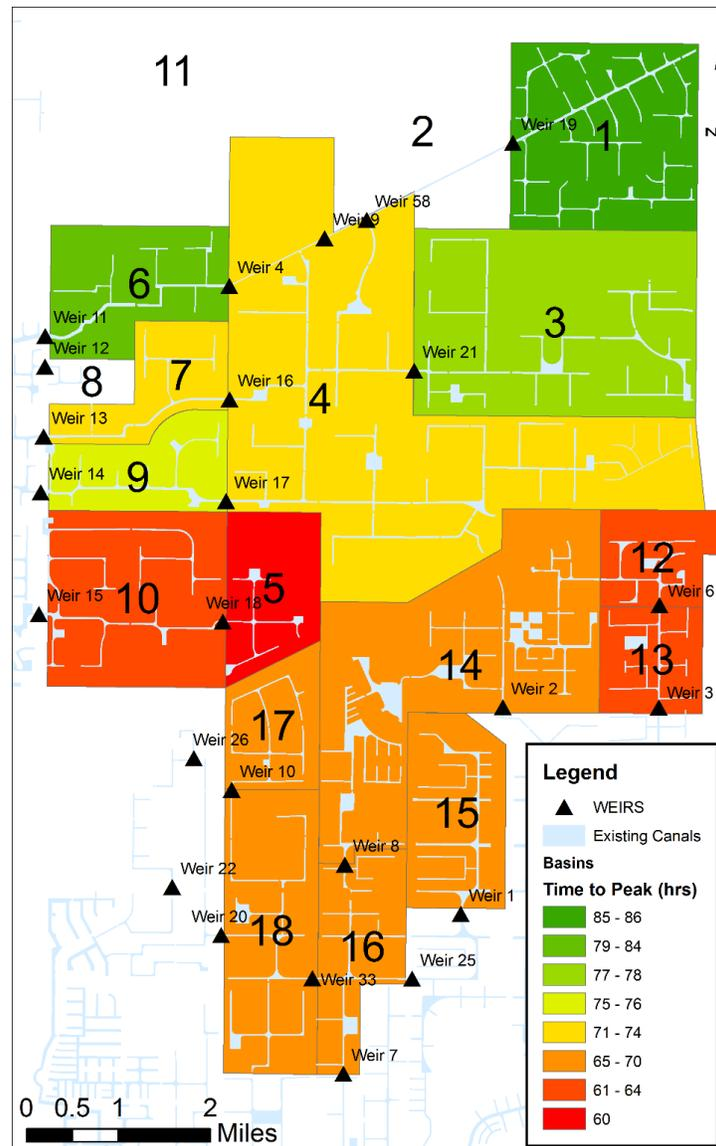
Figure 31. Map of the time to peak water elevation for critical Basins in the City of Cape Coral with existing structures and operations.
