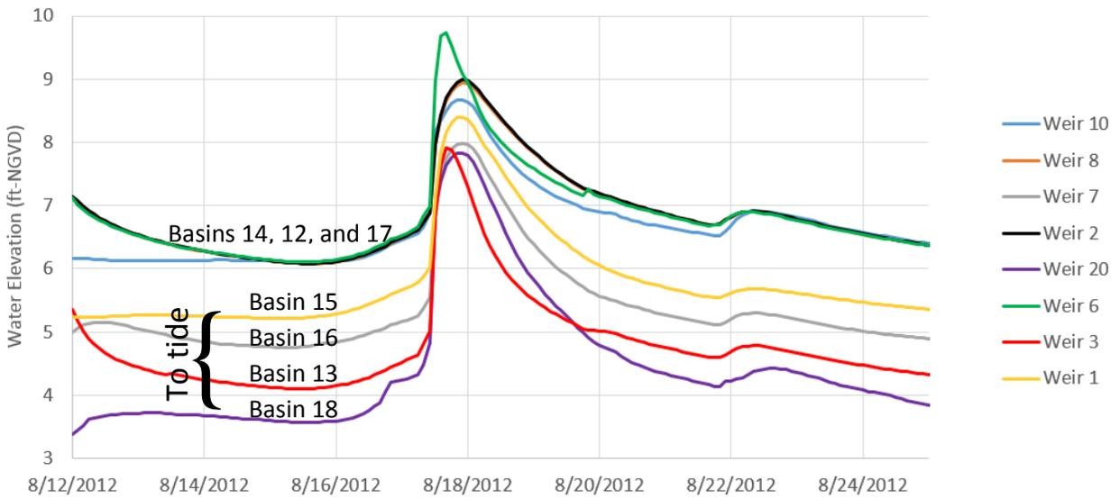
Figure 29. Hydrographs for the Lower Basins of Cape Coral for the first 13 days of the 25yr Design Storm simulation with Existing Conditions.
