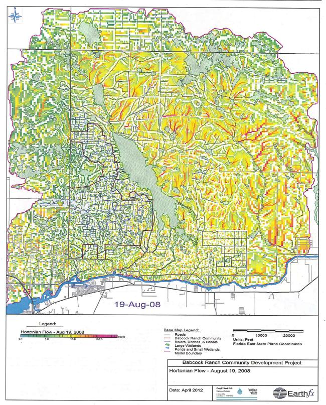
Figure 74: Simulated accumulated Hortonian flow (inches) for August 19, 2008.
