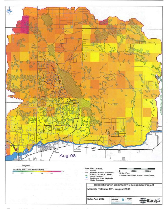
Figure 47: Monthly potential evapotranspiration (inches) in August 2008 under Current Conditions.
