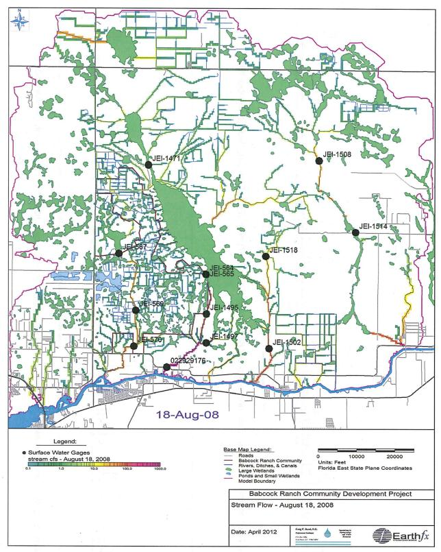
Figure 79: Simulated streamflow (cfs) for August 18, 2008 under Current Conditions.
