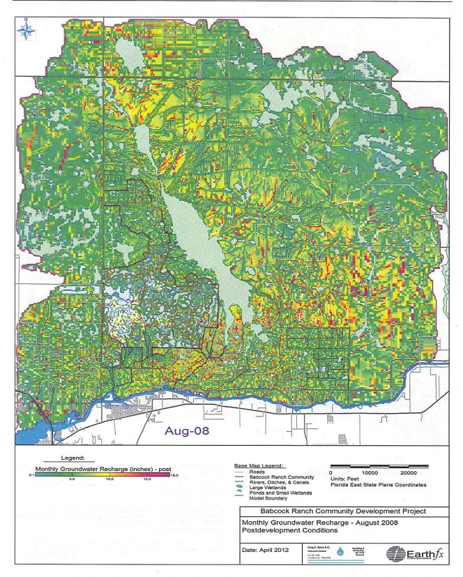
Figure 58: Monthly groundwater recharge (Infiltration - AET) in August 2008 under Postdevelopment Conditions.
