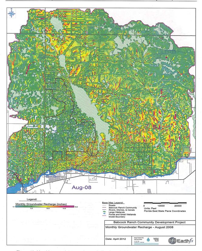
Figure 48: Monthly groundwater recharge (Infiltration - AET) in August 2008 under Current Conditions.
