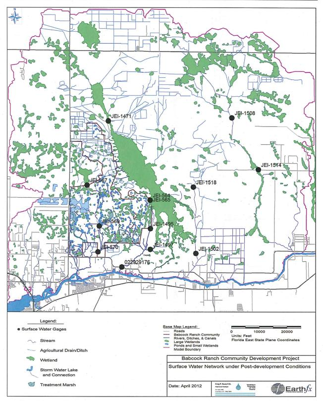
Figure 165: Surface water features represented in Post-development Conditions simulations.
