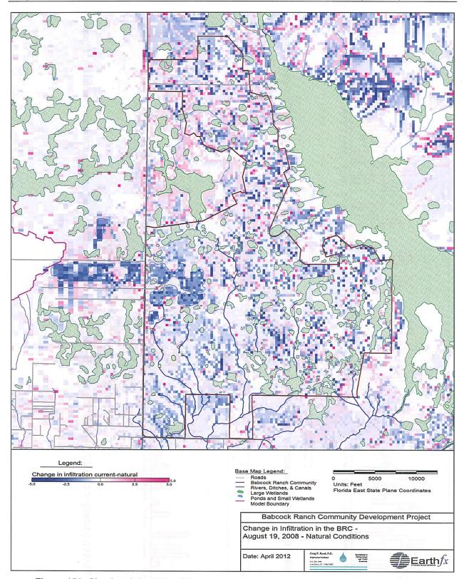
Figure 158: Simulated decrease (blue) and increase (red) in infiltration (Natural to Current Conditions) in the BRC on August 19, 2008.
