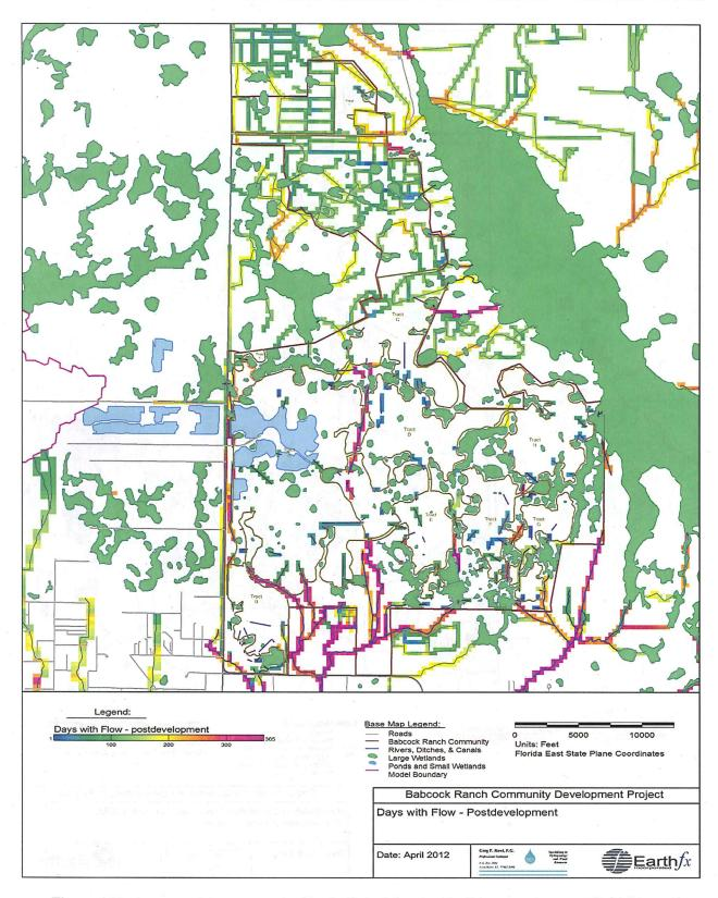
Figure 196: Average days per year with simulated flow under Post-development Conditions.
