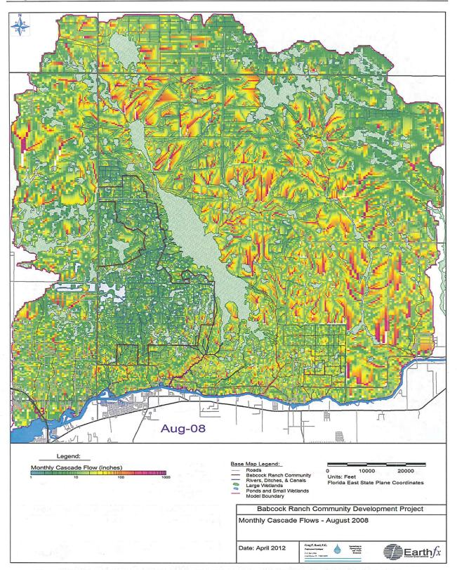
Figure 43: Monthly cascade flows (inches) for August 2008 (inches/month) under Current Conditions. Cascade flows include runoff generated and passing through each cell.
