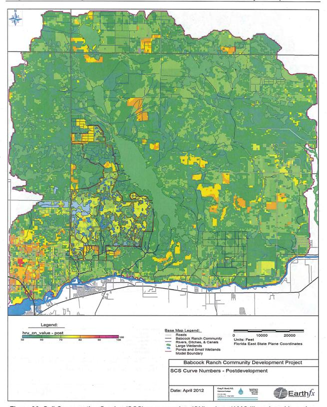
Figure 38: Soil Conservation Service (SCS) curve number (CN) values (AMC II) assigned based on combinations of soil type and Post-development Conditions land use. Wetland areas have no CN assigned.
