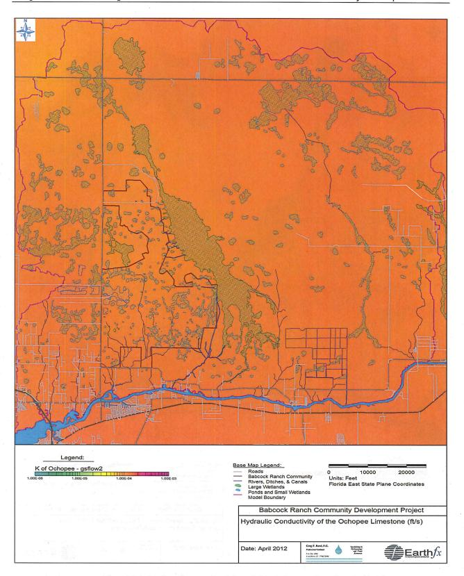
Figure 21: Hydraulic conductivity of the Ochopee limestone.
