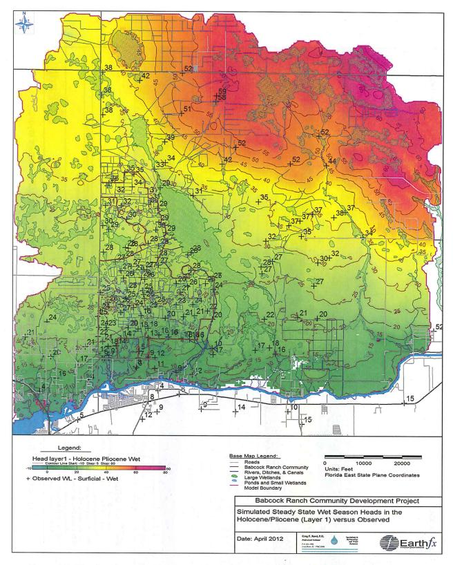
Figure 65: Simulated wet season steady-state heads (ft above NGVD) in the surficial aquifer.
