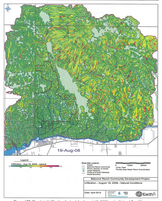
Figure 157: Simulated infiltration (inches) for August 19, 2008 under Natural Conditions.
