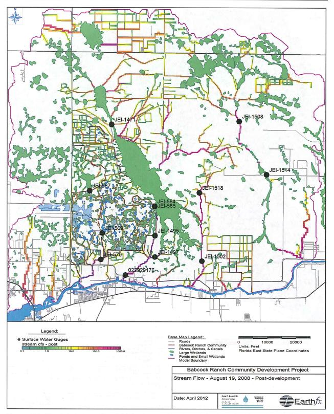
Figure 169: Simulated streamflow (cfs) for August 19, 2008 under Post-development Conditions
