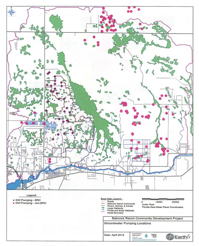
Figure 26: Location of pumping wells simulated in the model.
