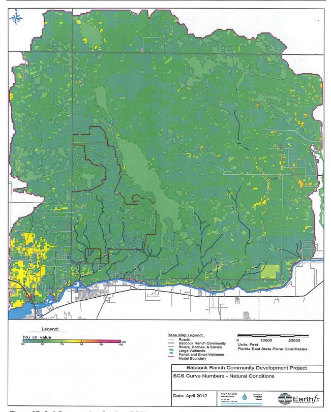
Figure 37: Soil Conservation Service (SCS) curve number (CN) values (AMC II) assigned based on combinations of soil type and Natural Conditions land use.
