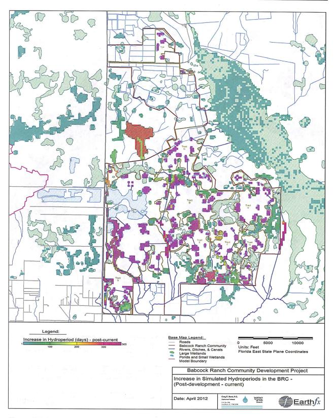
Figure 194: Increase in simulated hydroperiod (Post-development – Current Conditions) in the BRC.
