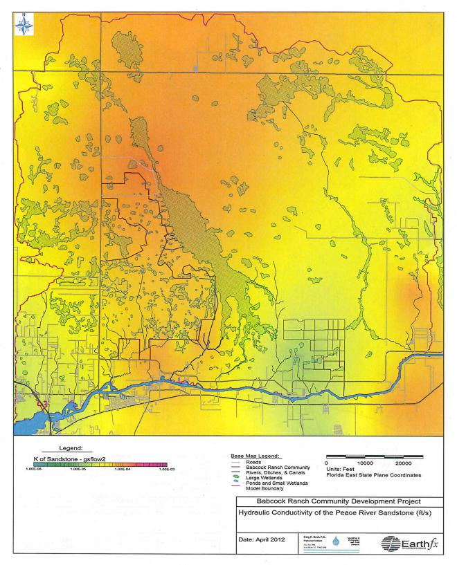
Figure 22: Hydraulic conductivity of the Peace River sandstone.
