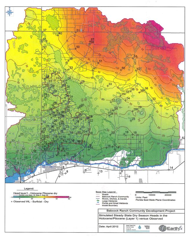
Figure 66: Simulated dry season steady-state heads (ft above NGVD) in the surficial aquifer.
