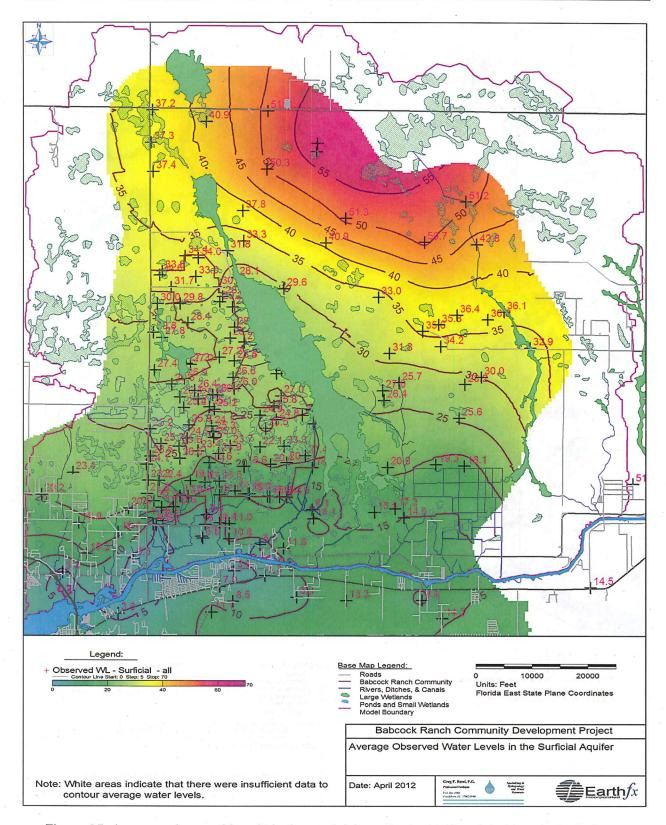
Figure 25: Average observed heads in the surficial aquifer and interpolated heads (in ft above NGVD).
