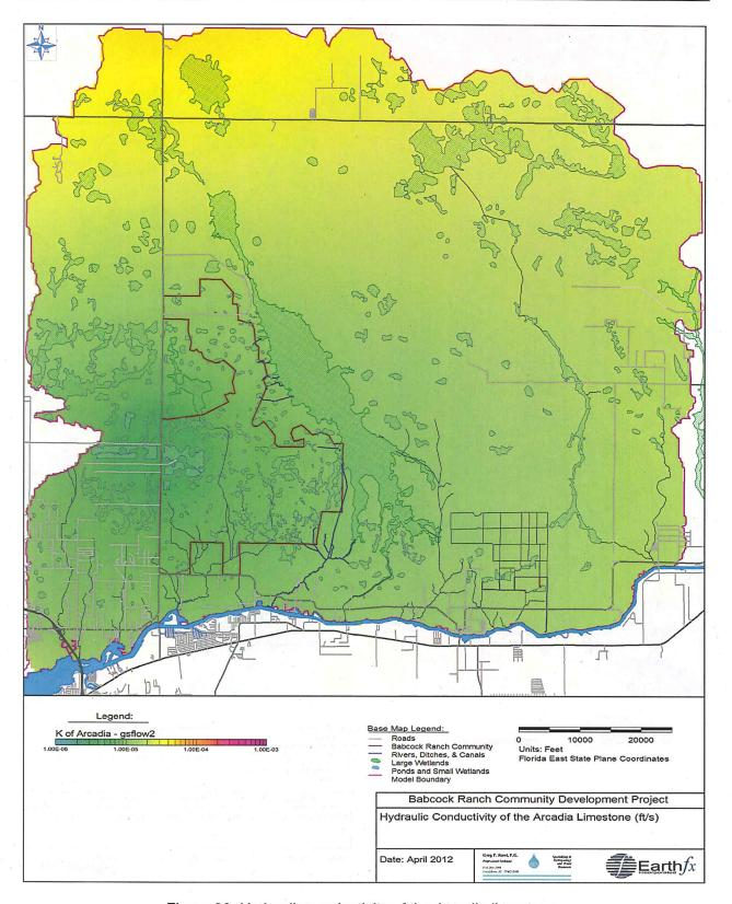
Figure 23: Hydraulic conductivity of the Arcadia limestone.
