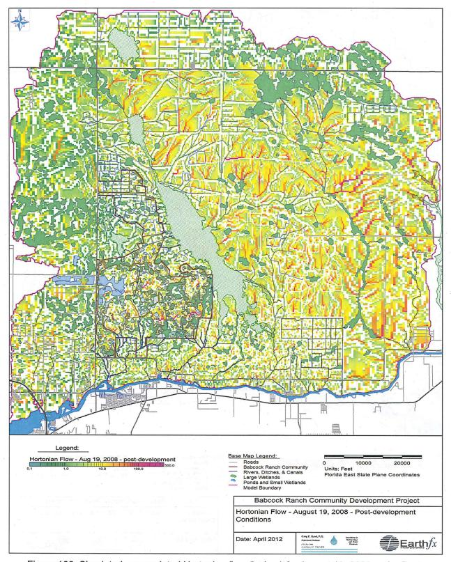
Figure 166: Simulated accumulated Hortonian flow (inches) for August 19, 2008 under Postdevelopment Conditions.
