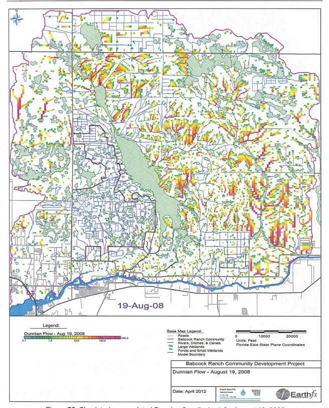
Figure 75: Simulated accumulated Dunnian flow (inches) for August 19, 2008
