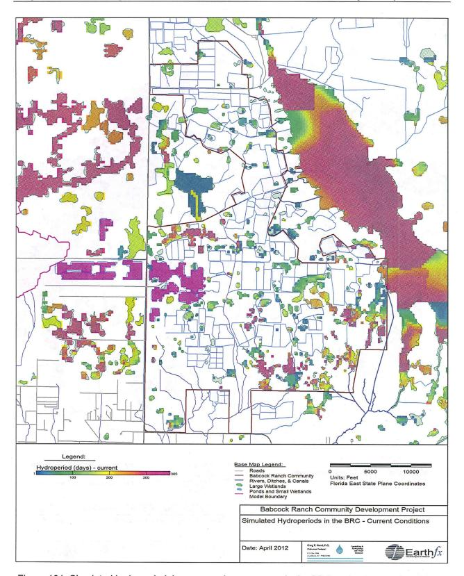
Figure 191: Simulated hydroperiod, in average days per year, in the BRC under Current Conditions.
