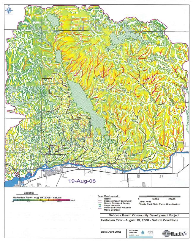
Figure 155: Simulated accumulated Hortonian flow (inches) for August 19, 2008 under Natural Conditions.
