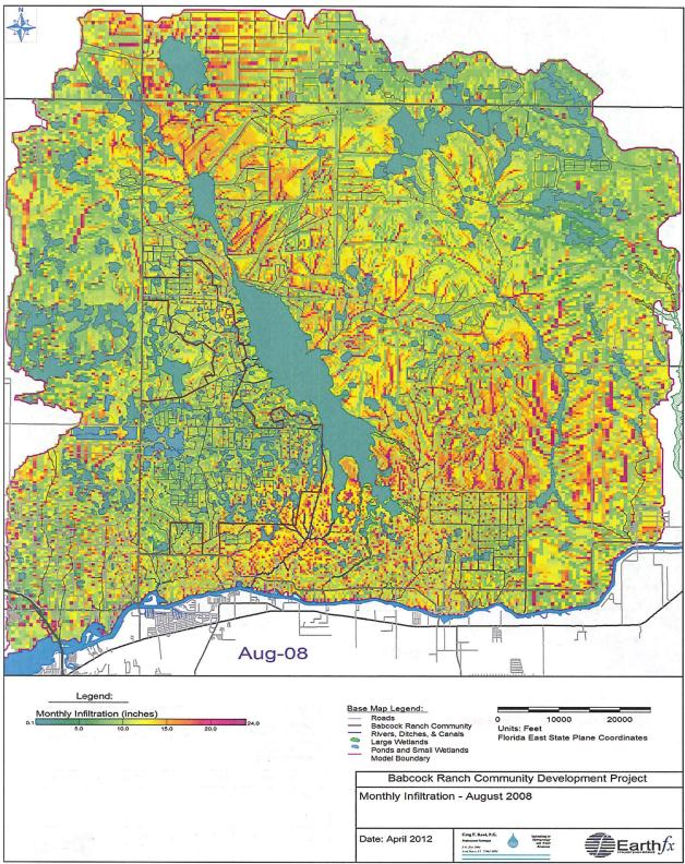
Figure 44: Monthly infiltration (inches) in August 2008 under Current Conditions.
