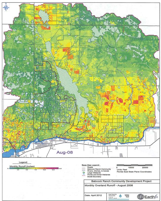
Figure 42: Monthly overland runoff (inches) in August 2008 under Current Conditions.
