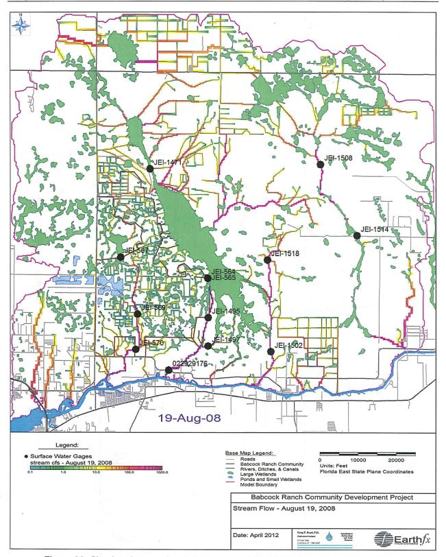
Figure 80: Simulated streamflow (cfs) for August 19, 2008 under Current Conditions.
