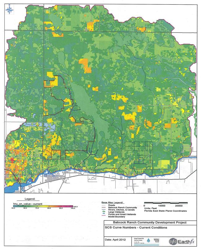
Figure 36: Soil Conservation Service (SCS) curve number (CN) values (AMC II) assigned based on combinations of soil type and Current Conditions land use. Wetland areas have no CN assigned.
