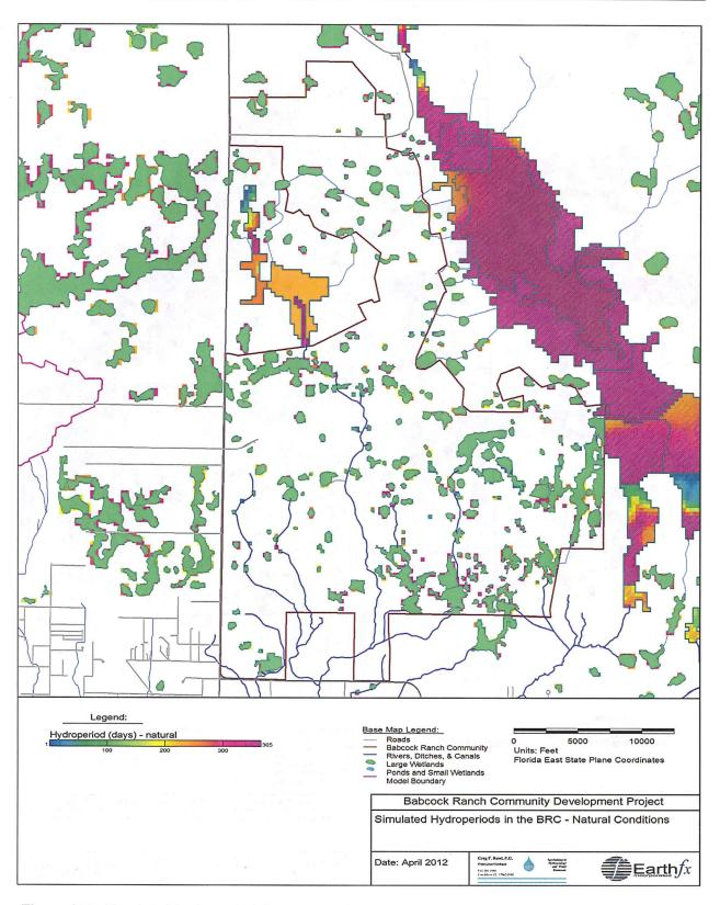
Figure 192: Simulated hydroperiod, in average days per year, in the BRC under Natural Conditions.
