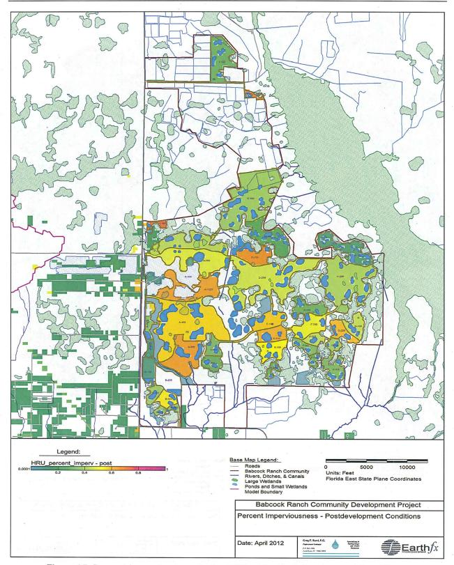
Figure 35: Percent imperviousness in the BRC under Post-development Conditions.
