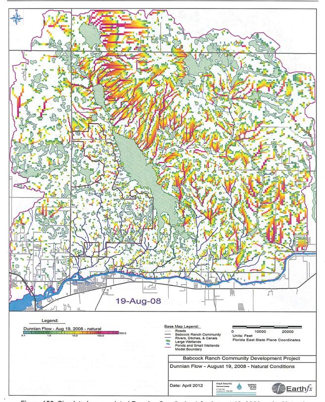
Figure 156: Simulated accumulated Dunnian flow (inches) for August 19, 2008 under Natural Conditions
