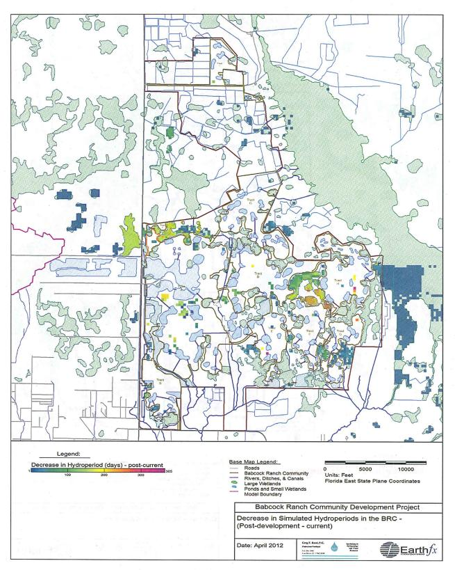
Figure 195: Decrease in simulated hydroperiod (Post-development – Current Conditions) in the BRC.
