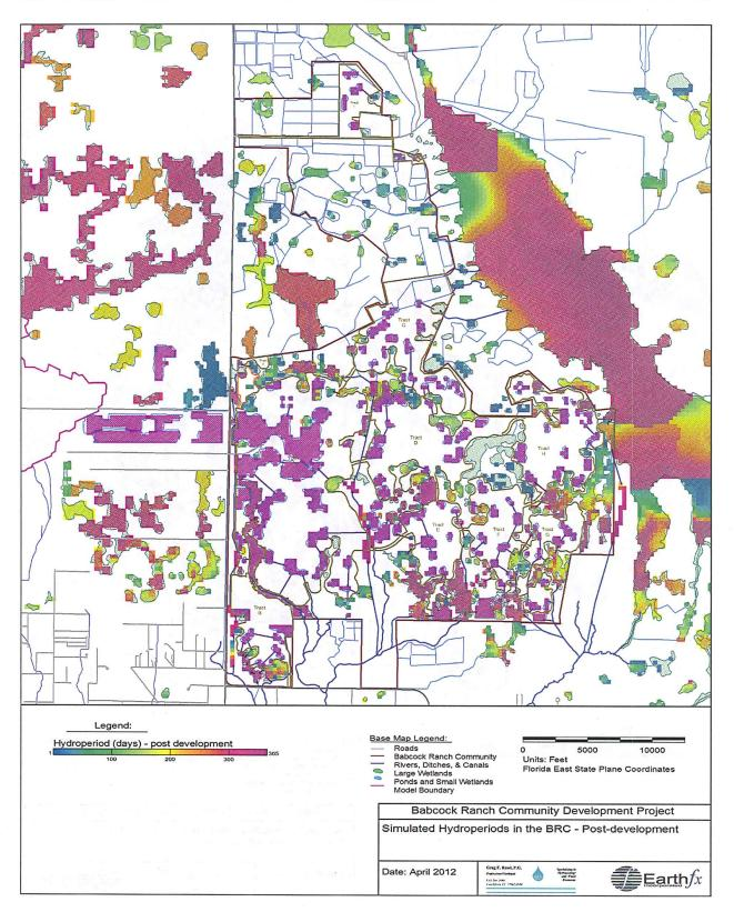
Figure 193: Simulated hydroperiod, in average days per year, in the BRC under Post-development Conditions.
