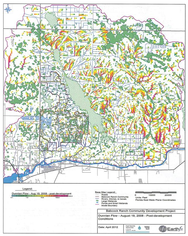
Figure 167: Simulated accumulated Dunnian flow (inches) for August 19, 2008 under Postdevelopment Conditions.
