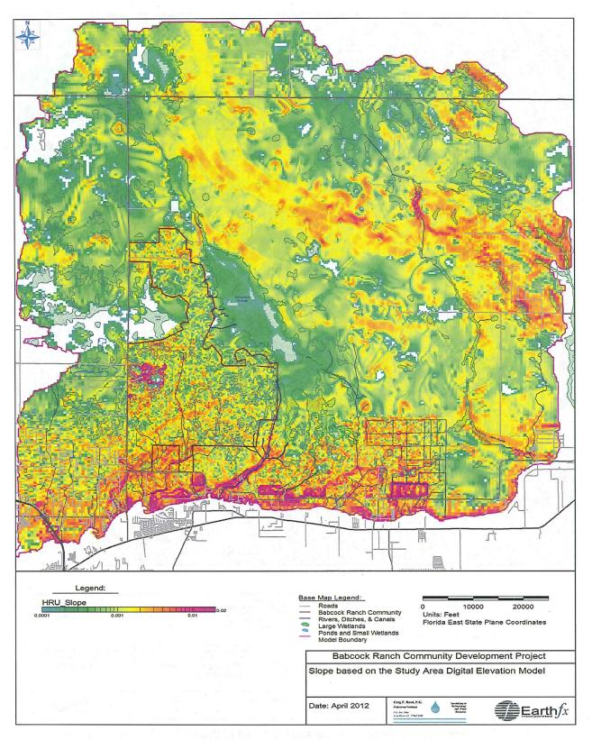
Figure 31: Slope values (decimal fraction) used in the PRMS model.
