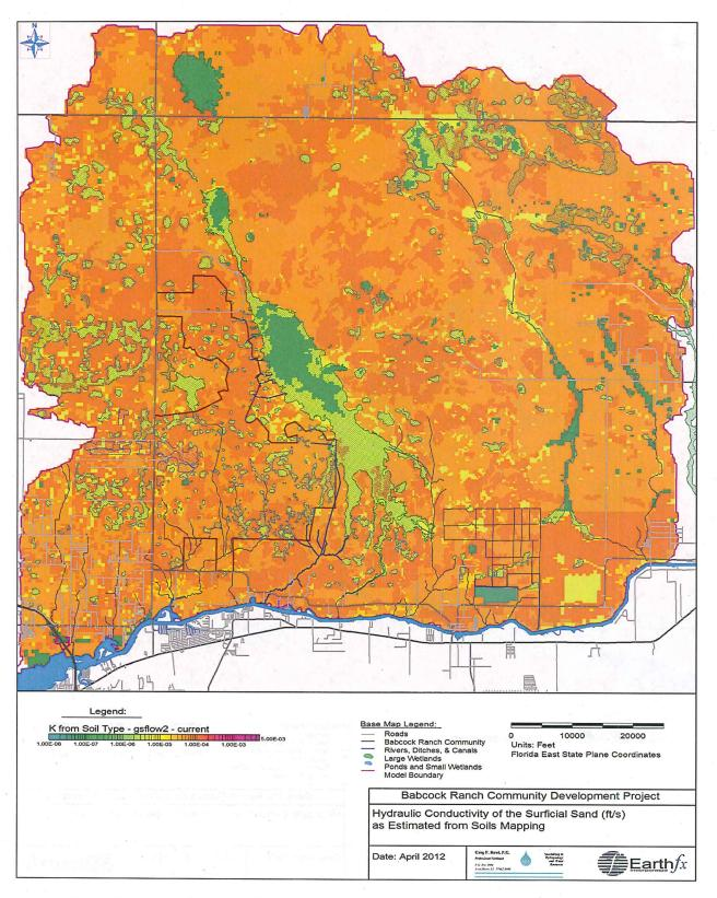
Figure 20: Hydraulic conductivity of the surficial sand as estimated from soils mapping.
