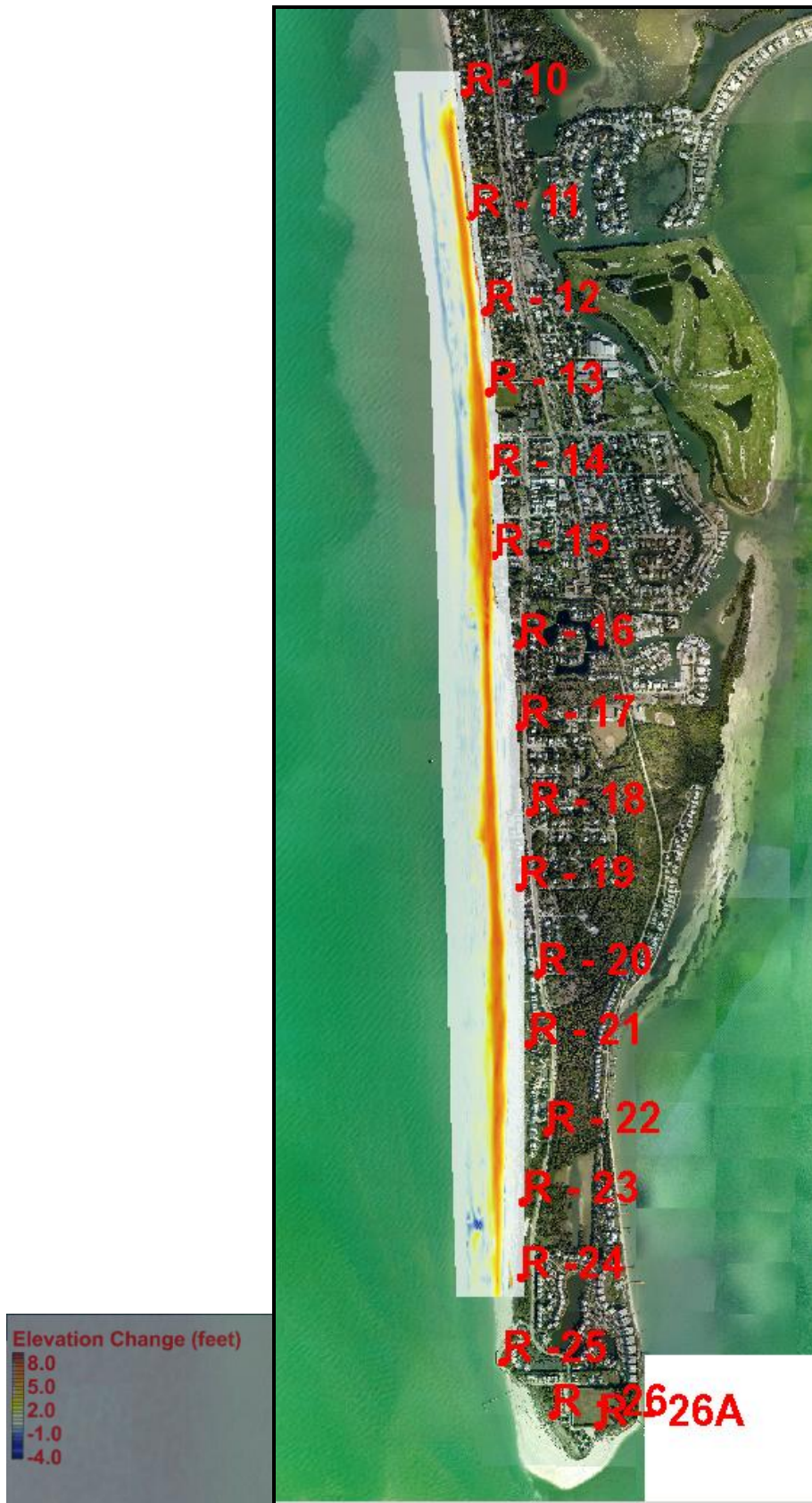
Figure 2. Limits of the 2013 renourishment construction project fill area depicted by elevation change and DNR survey monuments along Lee County Gasparilla Island Segment SPP.
