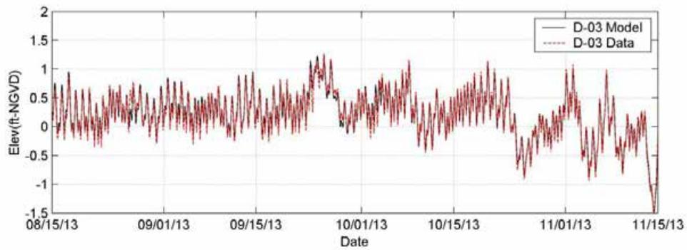
Figure 4-2a. Simulated vs Measured Water Level at Stations D-01 and D-03 (08/15/13 – 11/15/13)
