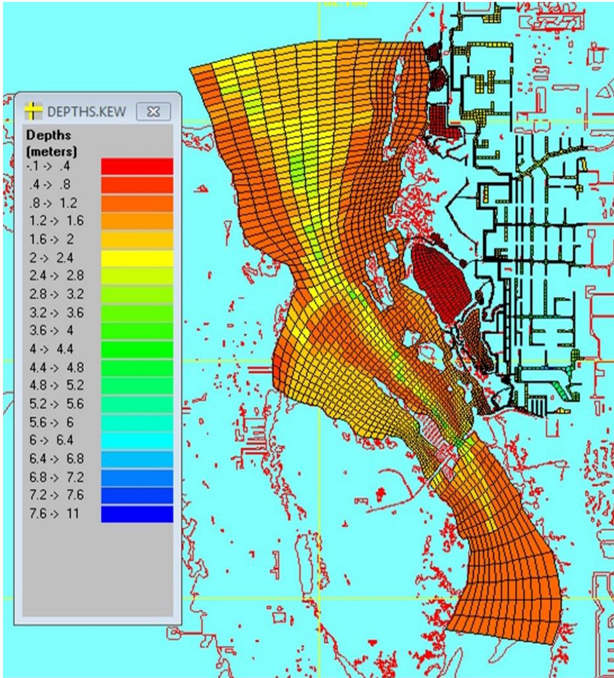
Figure 4-1. Model Grid and Bathymetry
