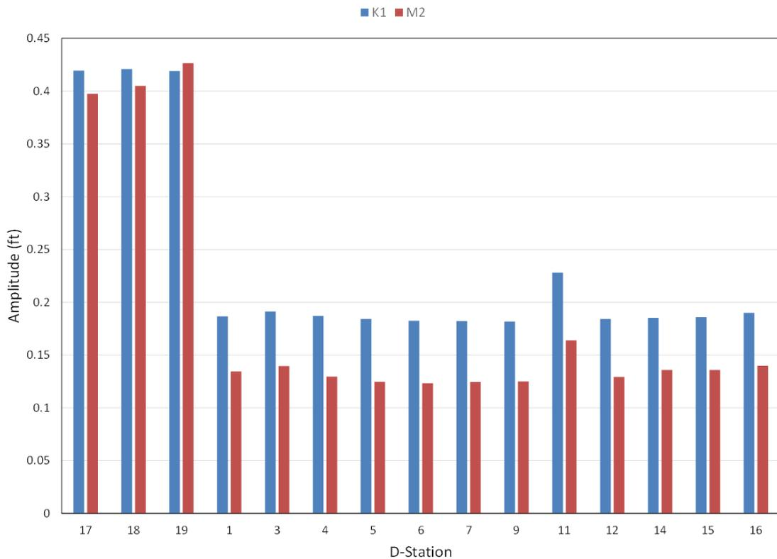
Figure 3-8a. Tidal Harmonic Amplitudes by Station
