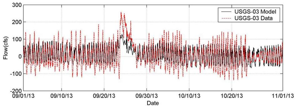
Figure 4-3b. Simulated vs Measured Flow at Stations USGS-02 and USGS-03 (09/01/13 – 11/01/13)
