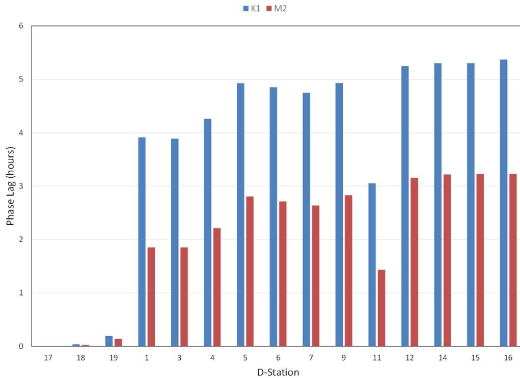
Figure 3-8b. Tidal Harmonic Phase Lag from D-17 by Station
