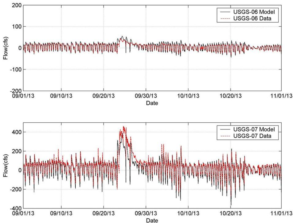
Figure 4-3c. Simulated vs Measured Flow at Stations USGS-06 and USGS-07 (09/01/13 – 11/01/13)
