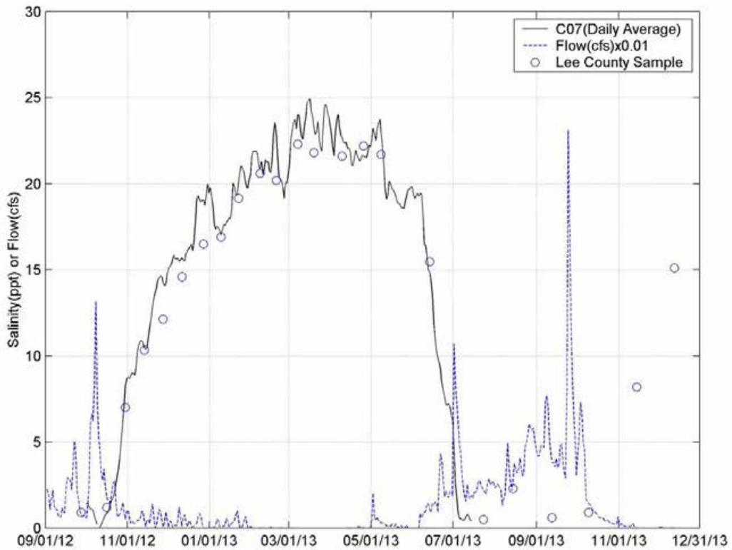
Figure 3-13b. Daily Average/Discrete Salinity versus Flow Over Weirs at C-07
