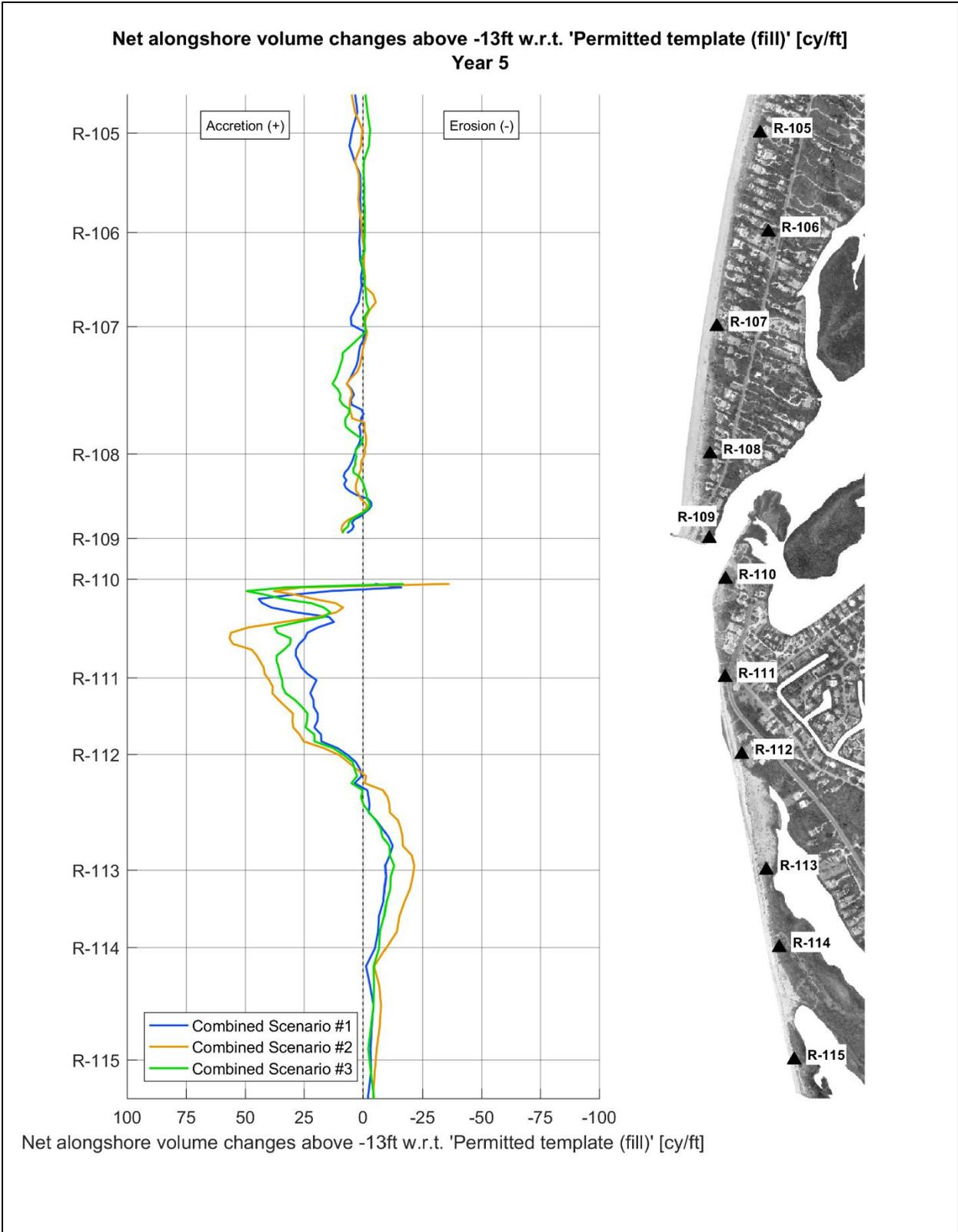
**Figure 3-4. Net alongshore volume changes relative to the permitted template (cy/ft).**
