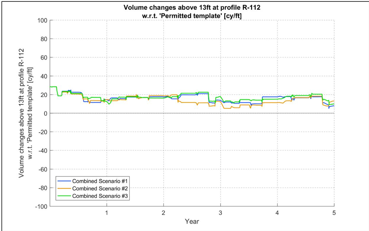
**Figure 3-7. Net volume changes at R-112 relative to the permitted template (cy/ft).**
