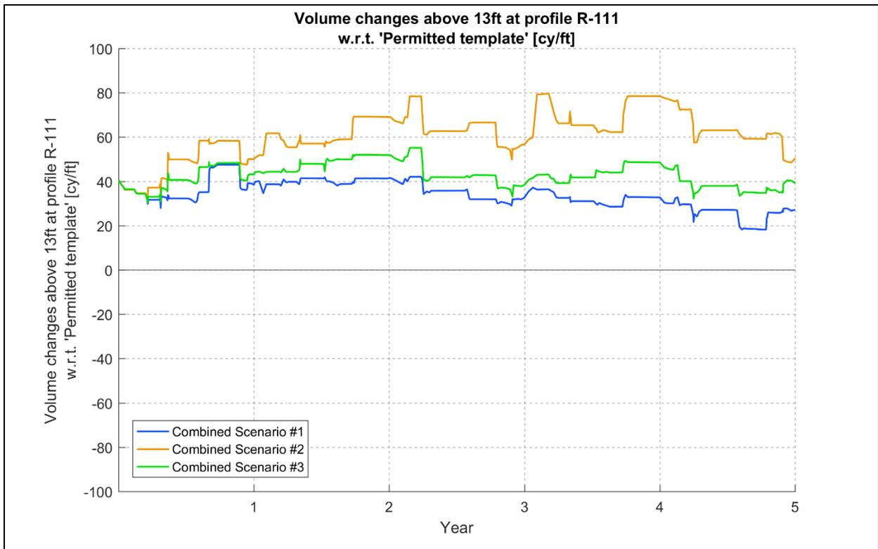
**Figure 3-6. Net volume changes at R-111 relative to the permitted template (cy/ft).**
