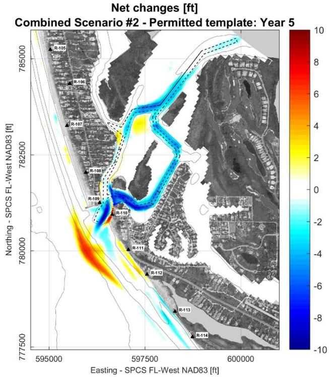
**Figure 3-2. Final Alternative 2 - net morphology changes relative to permitted template.**
