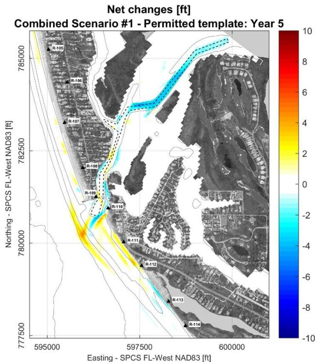
**Figure 3-1. Final Alternative 1 - net morphology changes relative to permitted template.**
