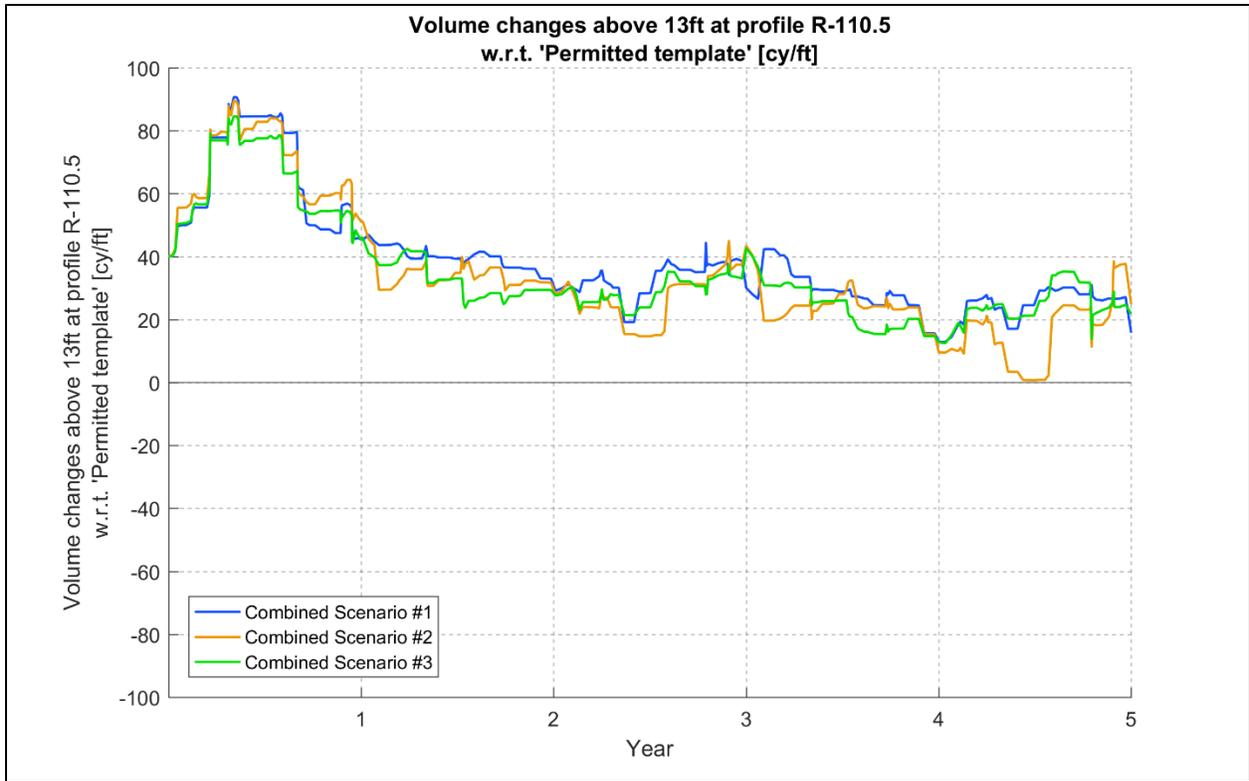
**Figure 3-5. Net volume changes at R-110.5 relative to the permitted template (cy/ft).**
