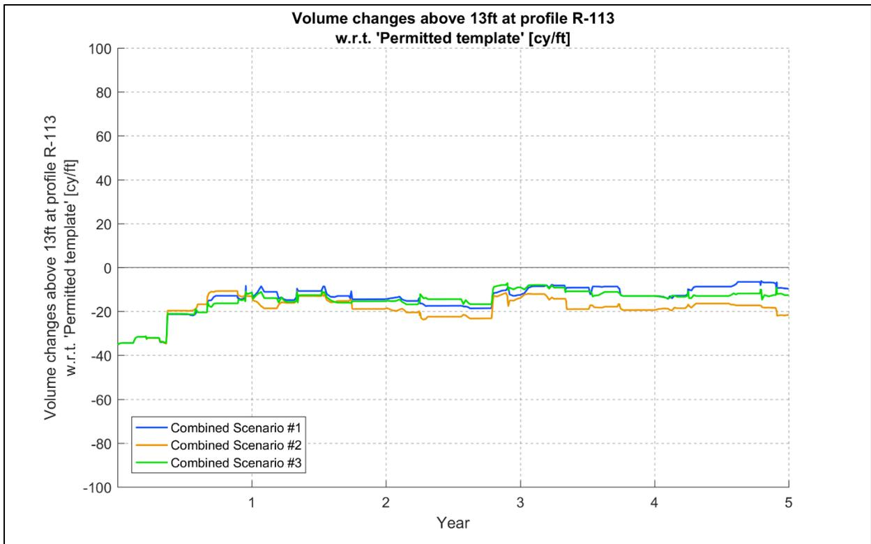
**Figure 3-8. Net volume changes at R-113 relative to the permitted template (cy/ft).**
