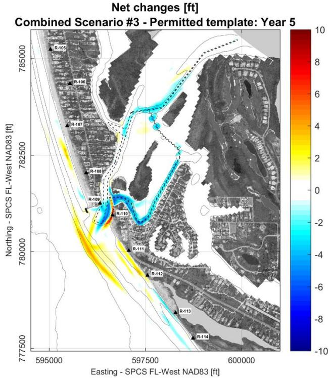
**Figure 3-3. Final Alternative 3 - net morphology changes relative to permitted template.**
