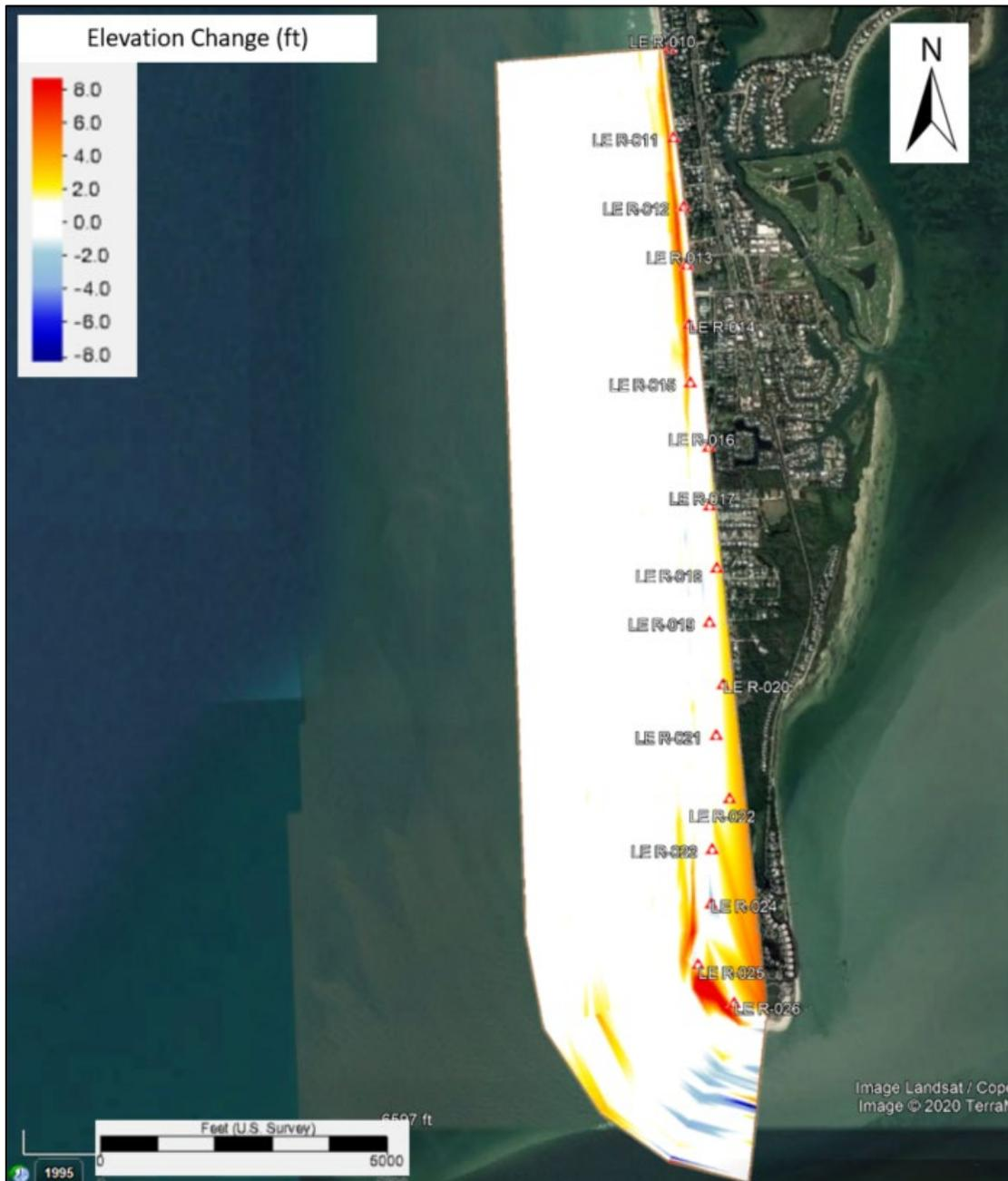
Figure 15: Elevation Change from Pre to Post-Construction Surveys
