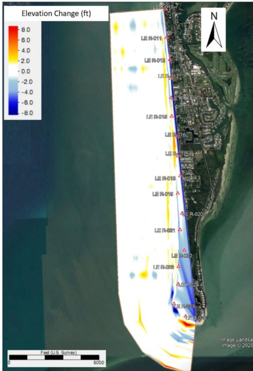
Figure 16: Elevation Changes between Post-Construction and Year 1 Monitoring Surveys
