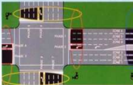
FULLY ACTUATED INTERSECTION SYSTEM DETECTION
