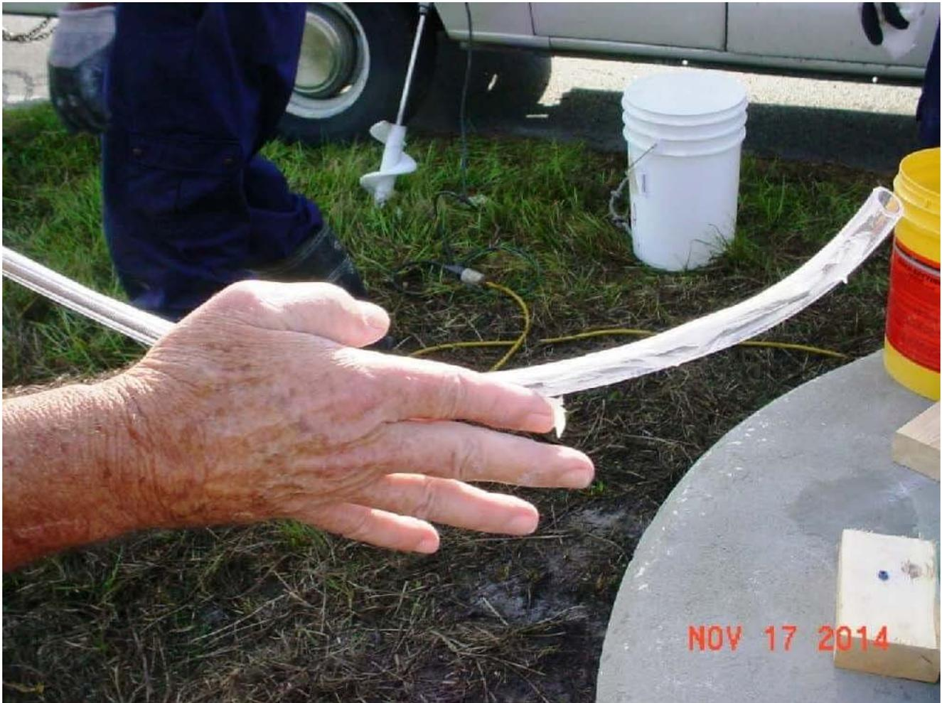
**The tube is then covered with petroleum based lubricant before it is reinstalled on the rod.**
