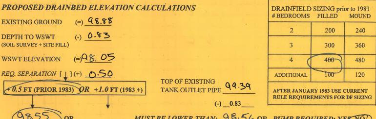
MUST BE LOWER THAN: 98.56 OR PUMP REQUIRED: YES NO OR NEW ELEV OF BOTTOM DB STONE)
