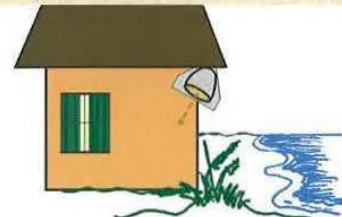
Rotate the light away from the beach. It may need additional shielding to prevent reflection off of the building.
