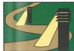
Use low profile lighting or low bollards with low wattage bulbs and 180° shields on the beach side.
