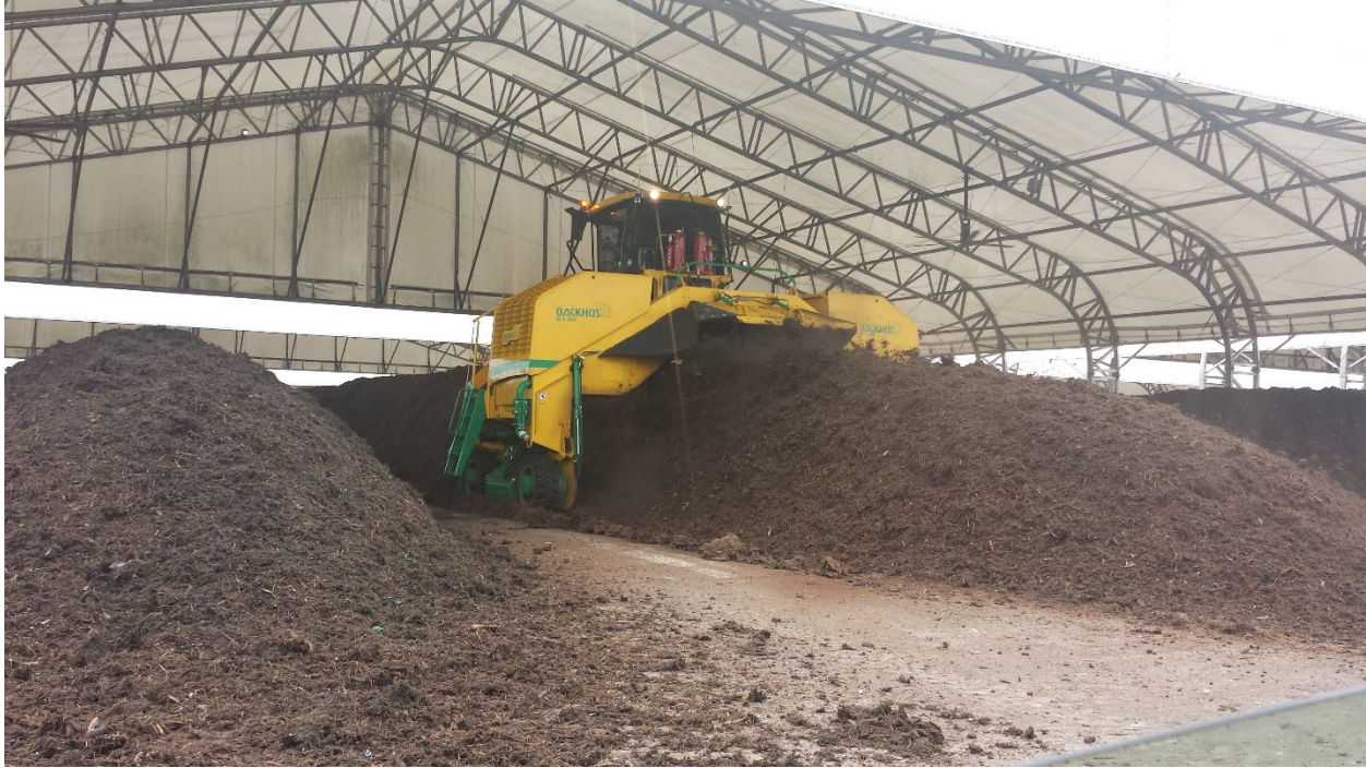
The County's composting facility utilizes specialized equipment, shown above, to periodically turn the mulch and sludge amendment to reduce heat buildup from bacteriological decomposition to more efficiently produce compost for resale. Link for brief demonstration: https://youtu.be/szRFHovcAIQ
