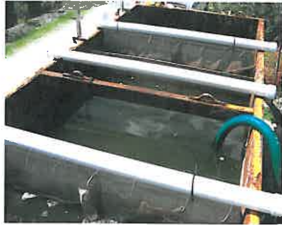
Photo 3: Pilot plant, top view. The white pvc has jute mat attached. The green piping is a dewatering pump suction line used to drain the tank after test runs. During the actual test runs an additional jute mat was hung at the rear of the tank.
