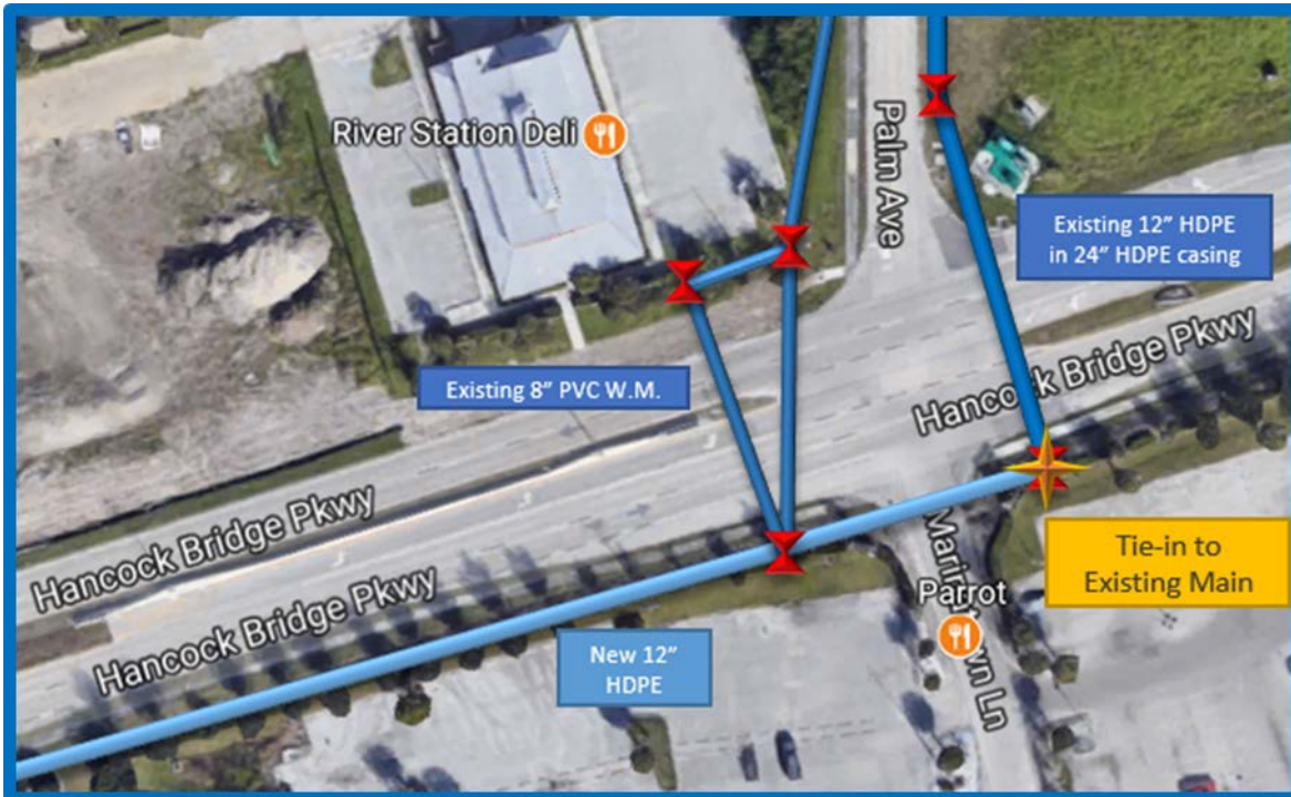
Figure 3-3: Replacement Pipe at Hancock Bridge Parkway and Palm Avenue
