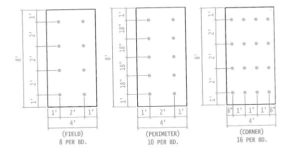
Induction Welded Insulation Attachment Patterns Provided by FiberTite
