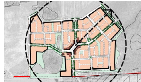
This illustrative site plan for a mixed-use community shows a quarter-mile radius which represents the five-minute walk that many people prefer to driving the same distance.
