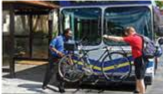
LeeTran has bike racks mounted on the front of every bus and trolley.
