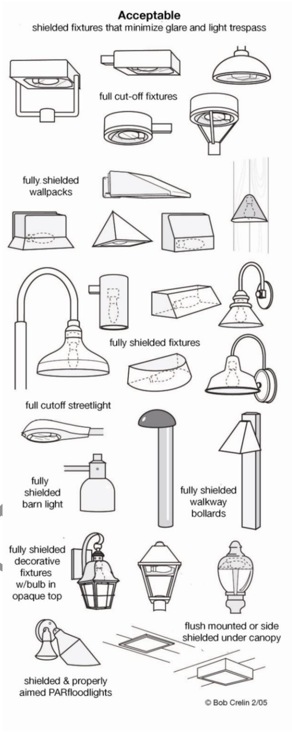
Figure 3: Examples of acceptable fixtures
