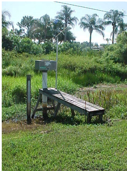
USGS Streamgage Located at the Confluence of Gator Slough Channel and East Side Ditch of US-41
