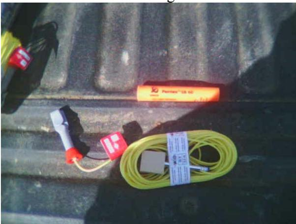
Non-electric detonator and primer cartridge
