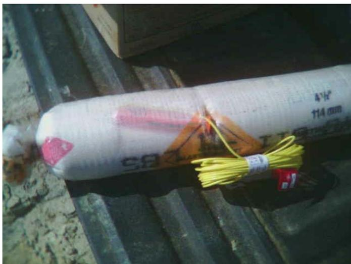
Emulsion cartridge with detonator & primer charge
