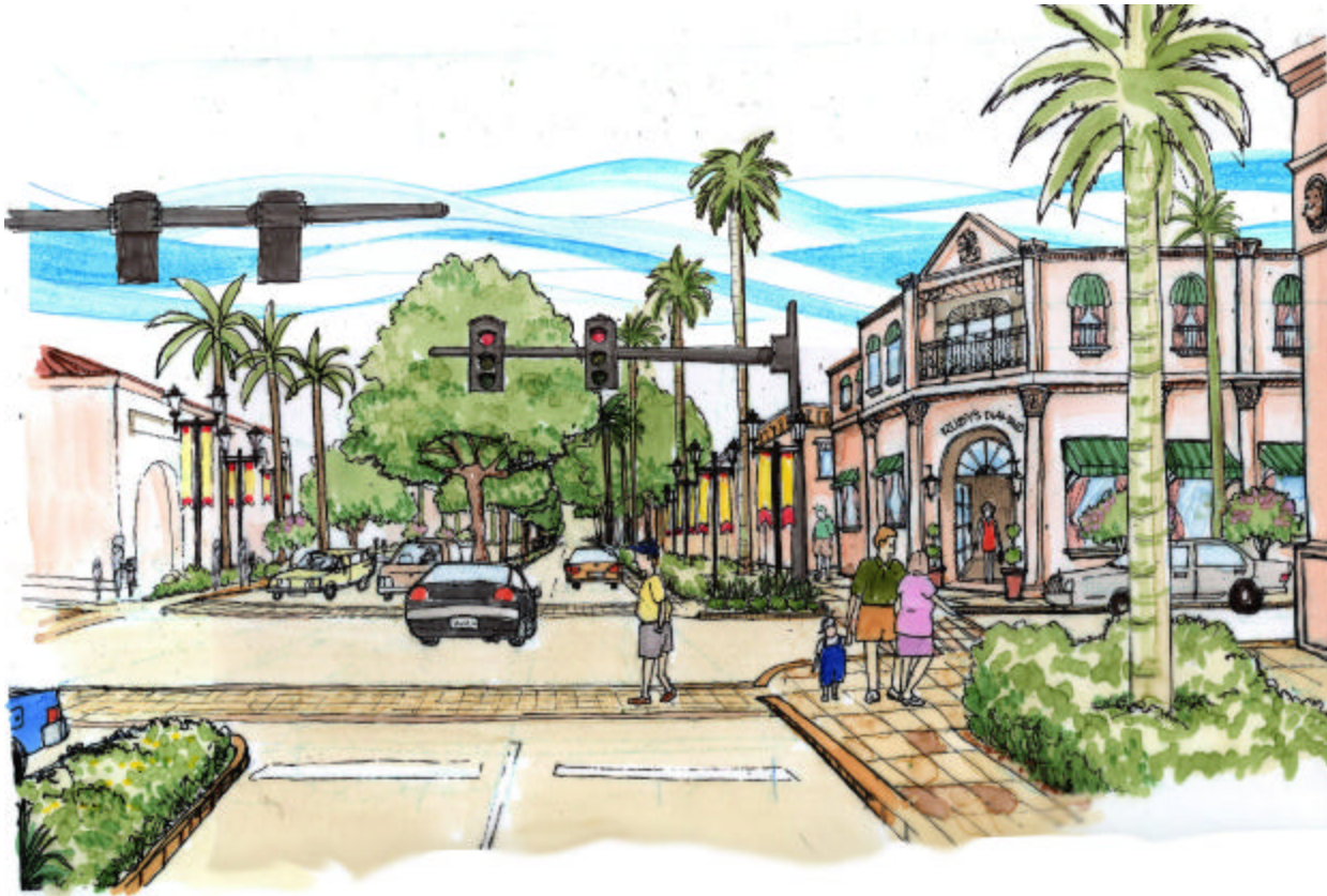
Rendering of Commercial Node with enhanced landscaping, a median, sidewalk, crosswalk pavers, and the buildings located at the roadway to create a pedestrian oriented environment
