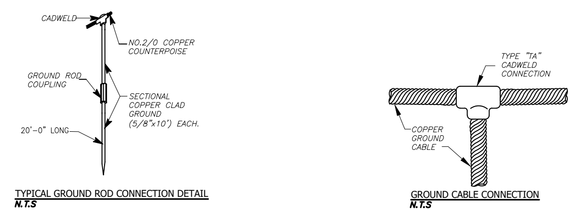
TYPICAL GROUND ROD CONNECTION DETAIL N.T.S.
